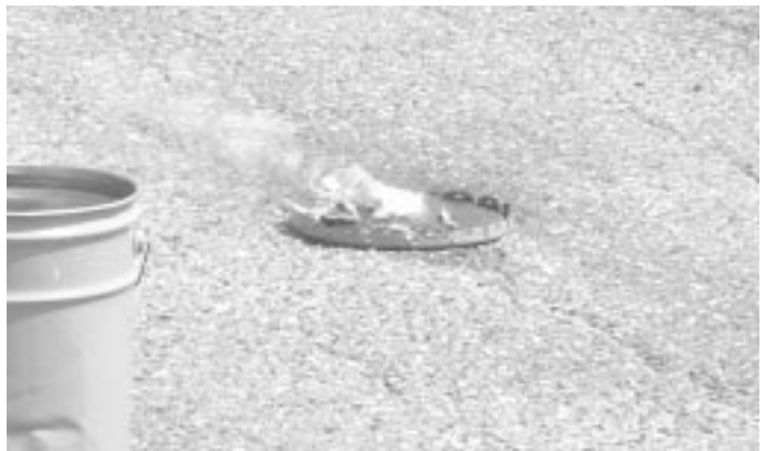
Photo 2 – Small quantity of lithium burns very intensely.
