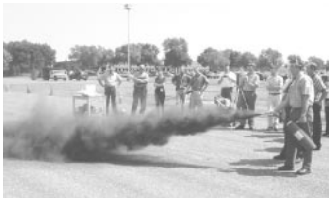
Photo 4 – Application of specialized extinguishing agent (note the darker gray/brown color of the agent).
