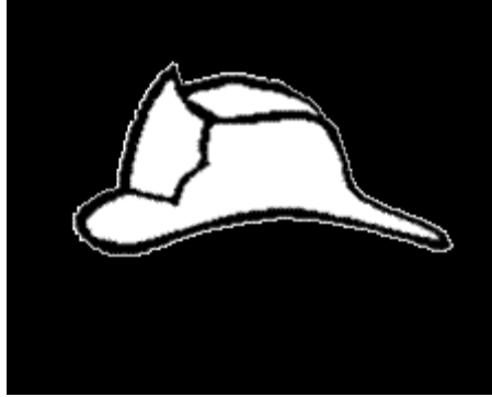
Figure 54.12.10 First Responders Use Elevator Symbol
