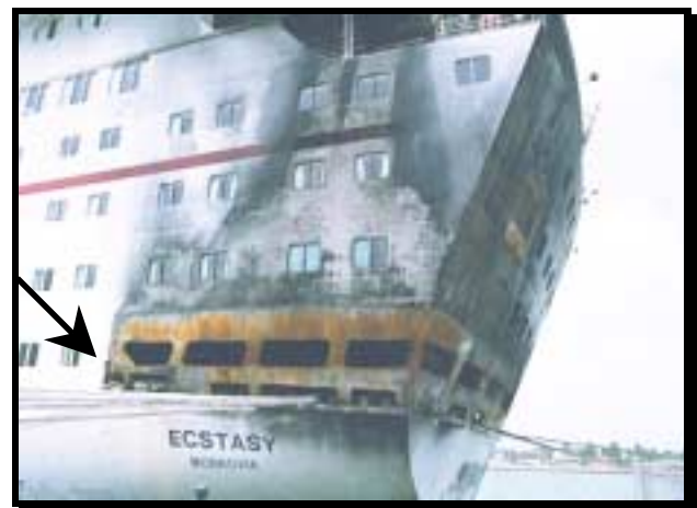
Photo showing damage on the port side of the ship, outside the mooring deck. The arrow shows the location of the bulkhead where the fire brigade held the fire's spread. (NFPA)
