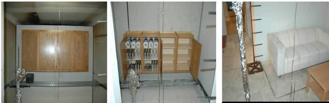
Figure 2: Photograph of elevated cabinet array (left), floor-level cabinet array (middle), and upholstered sofa (right) fire test setups.
