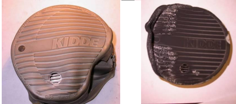
Figure 4: Photographs illustrating the different levels of soot deposited on alarms exposed to varying fire conditions.
