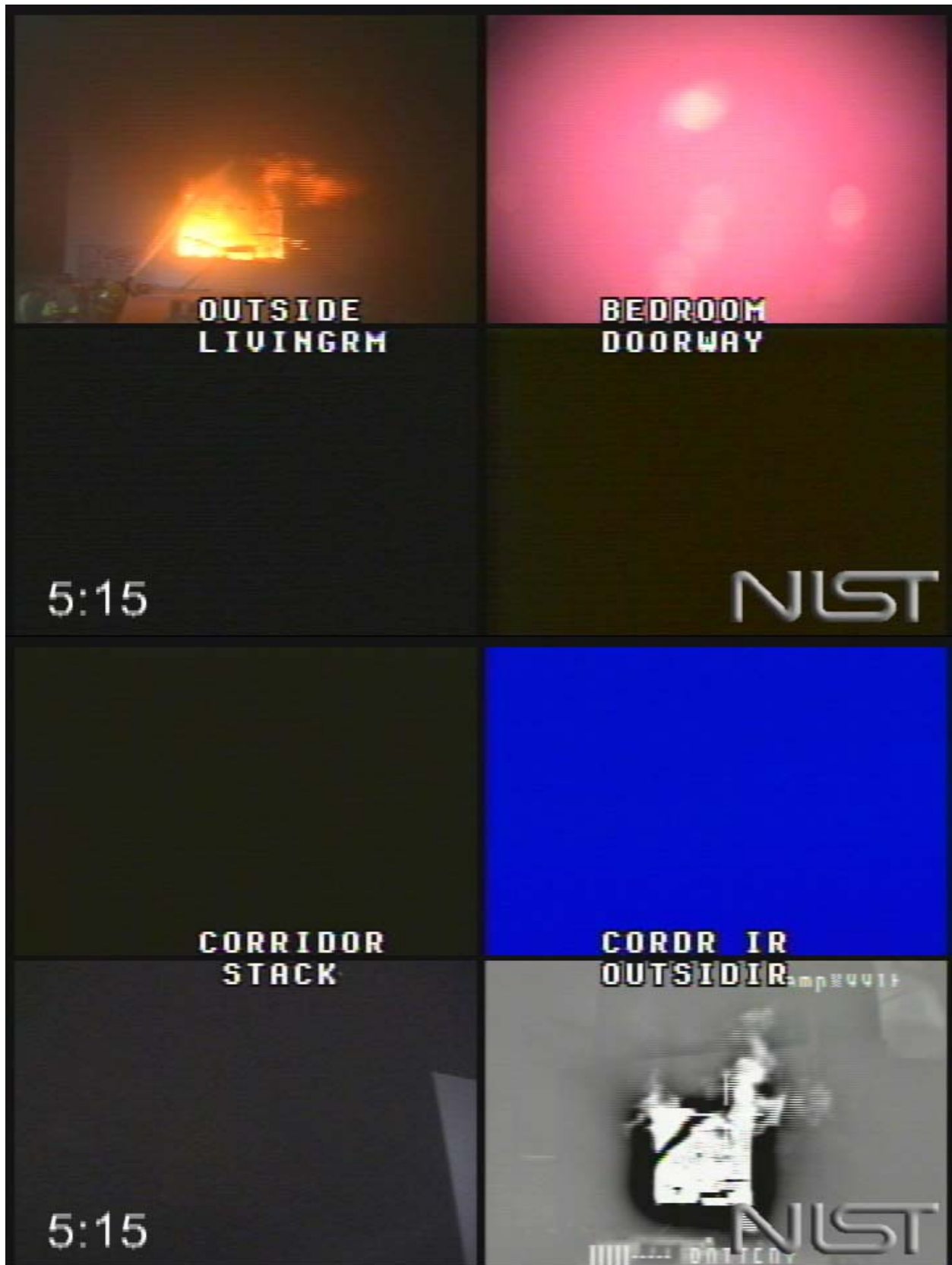
Figure 5.8.1-10. Experiment 8, flames withdraw from vent, 315 s after ignition.
