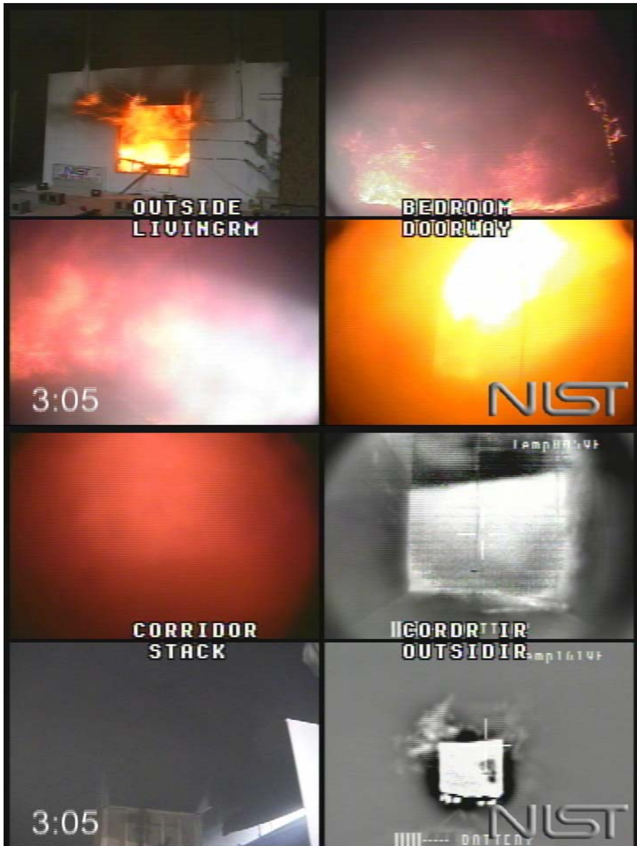
Figure 5.8.1-6. Experiment 8, corridor flames, 185 s after ignition.
