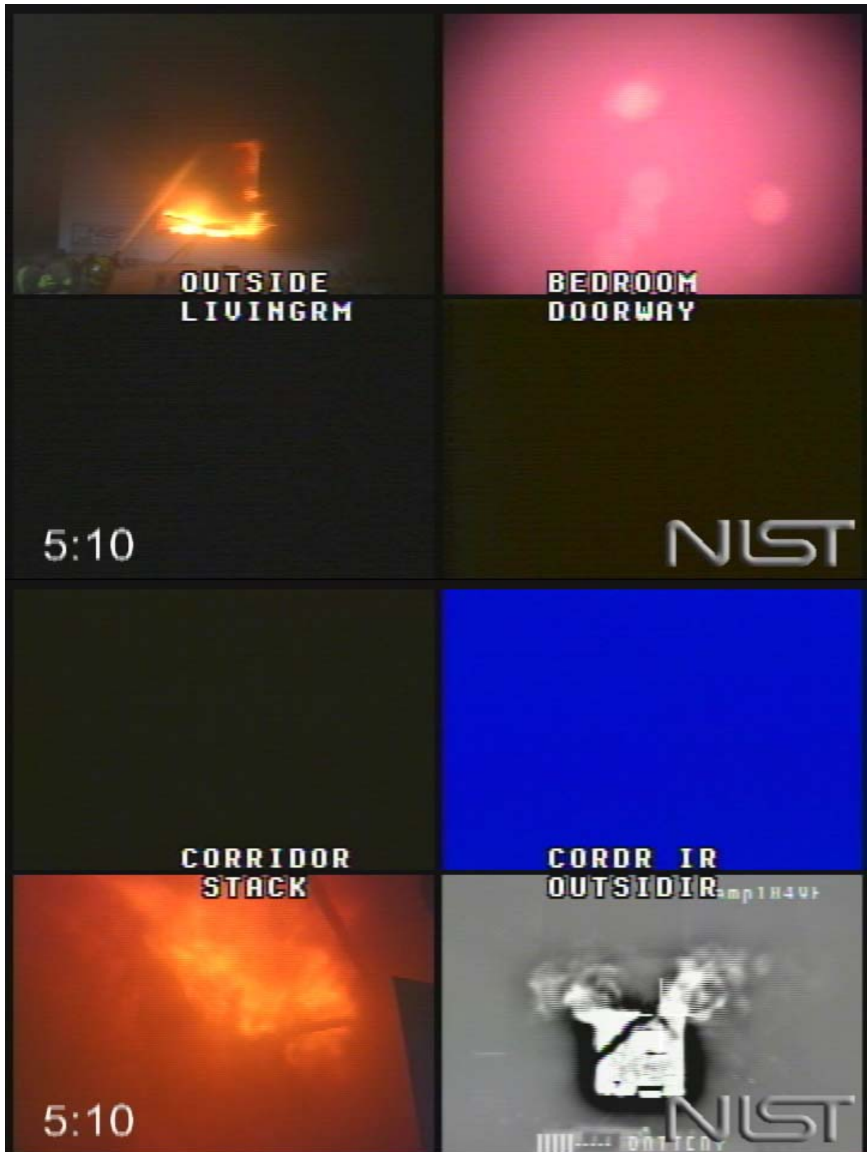
Figure 5.8.1-9. Experiment 8, indirect suppression started, 310 s after ignition.
