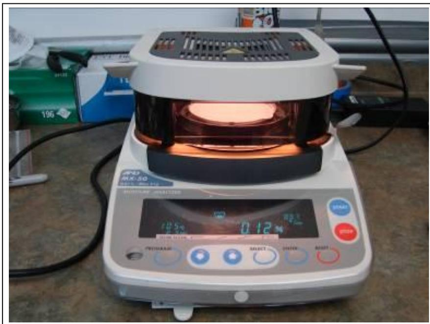
**FIGURE 6. Moisture analyzer used to measure the moisture content of the dried cellulose powder.**
