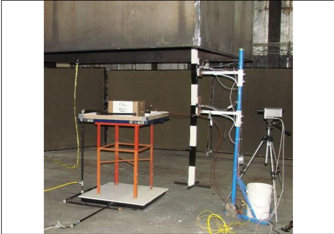
FIGURE 1. Photograph showing an overview of 2MW hood and the test set up and instrumentation under the hood.
