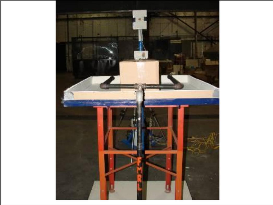
FIGURE 4. Profile of the burner and carton with test material centered on the tray and load cell.
