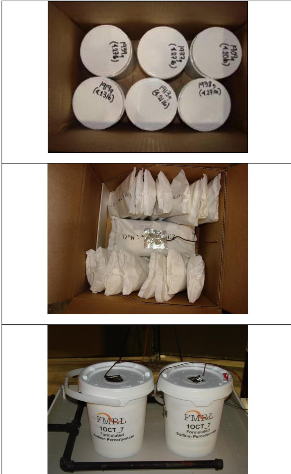
FIGURE 5. Combustible test packaging consisting of 6 HDPE containers in a DW carton(top). Other packaging evaluated were twenty four 1-lb bags in a DW carton (middle) and 2.5 gallon HDPE pails (bottom).
