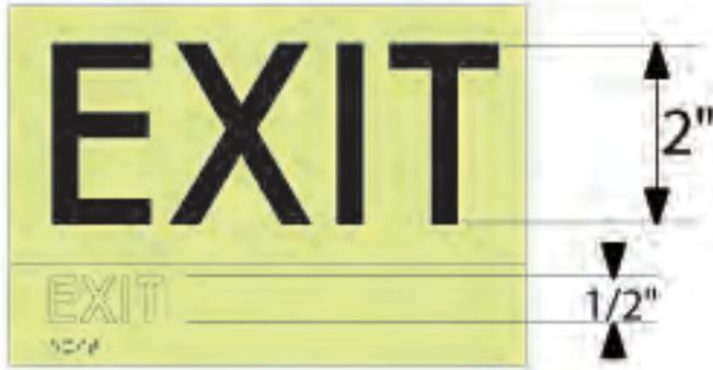
This is a drawing of a photoluminescent visual exit sign that could be mounted next to a door (or separately, on the door) and it is accompanied by the new “invisible” raised characters and braille that are especially easy for a completely blind person to read. This concept might also be used on a low level sign.
