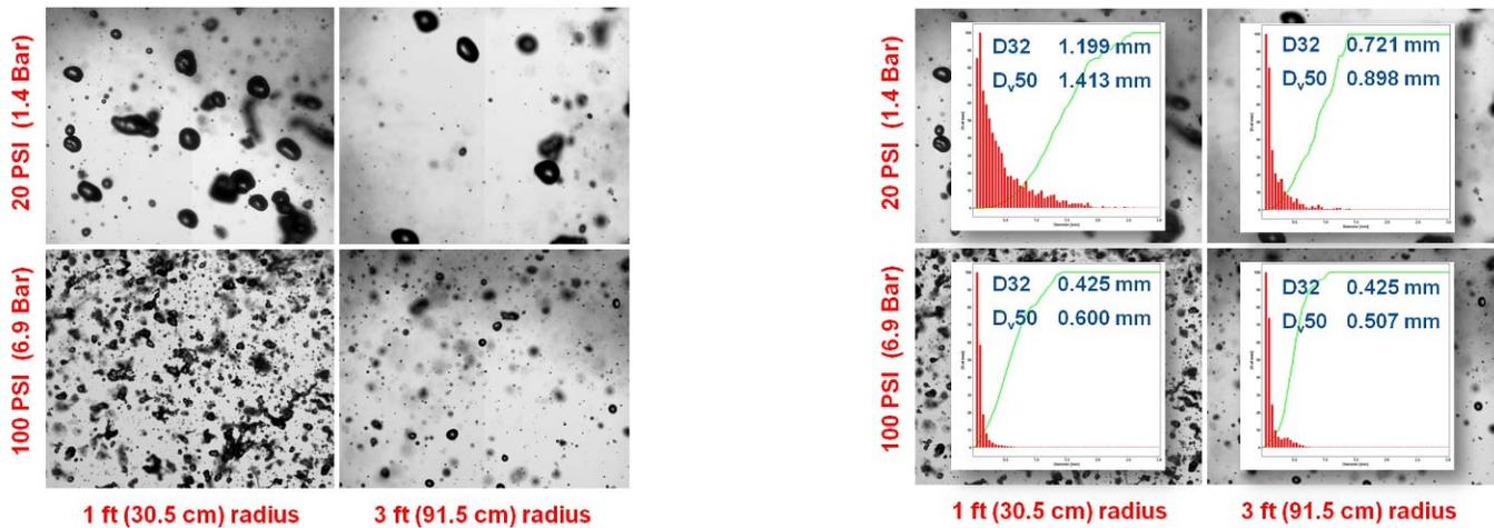
If only the K-factor is changed, the increase in K-factor from 1.2K (K17.3) to 3K (K43.2) in general caused an increase in the D32 and DV50 values. For example, as the K-factor increases (and the pressure is held constant), there is more water that must be pushed through the same area resulting in a thicker water sheet and subsequently larger droplets.
