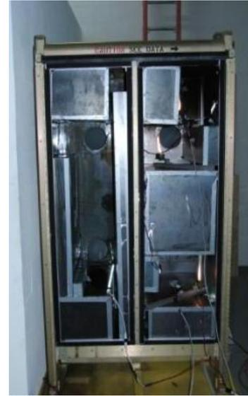
**Figure 2. ISS obstructed rack replica (shown here without front panel).**
