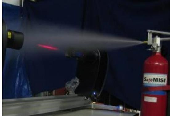
**Figure 1. ADA Technologies prototype FWM extinguisher.**
