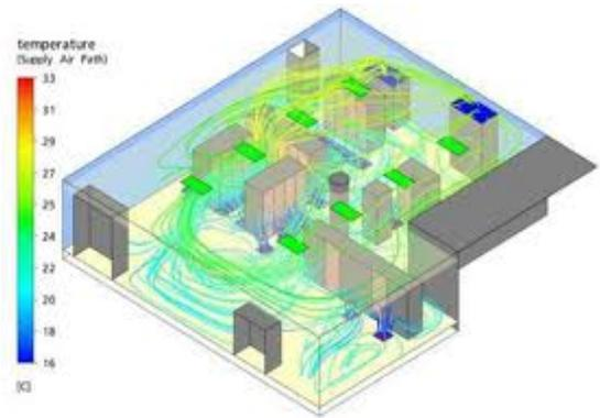
Figure 4 – CFD model of airflow in a data center
