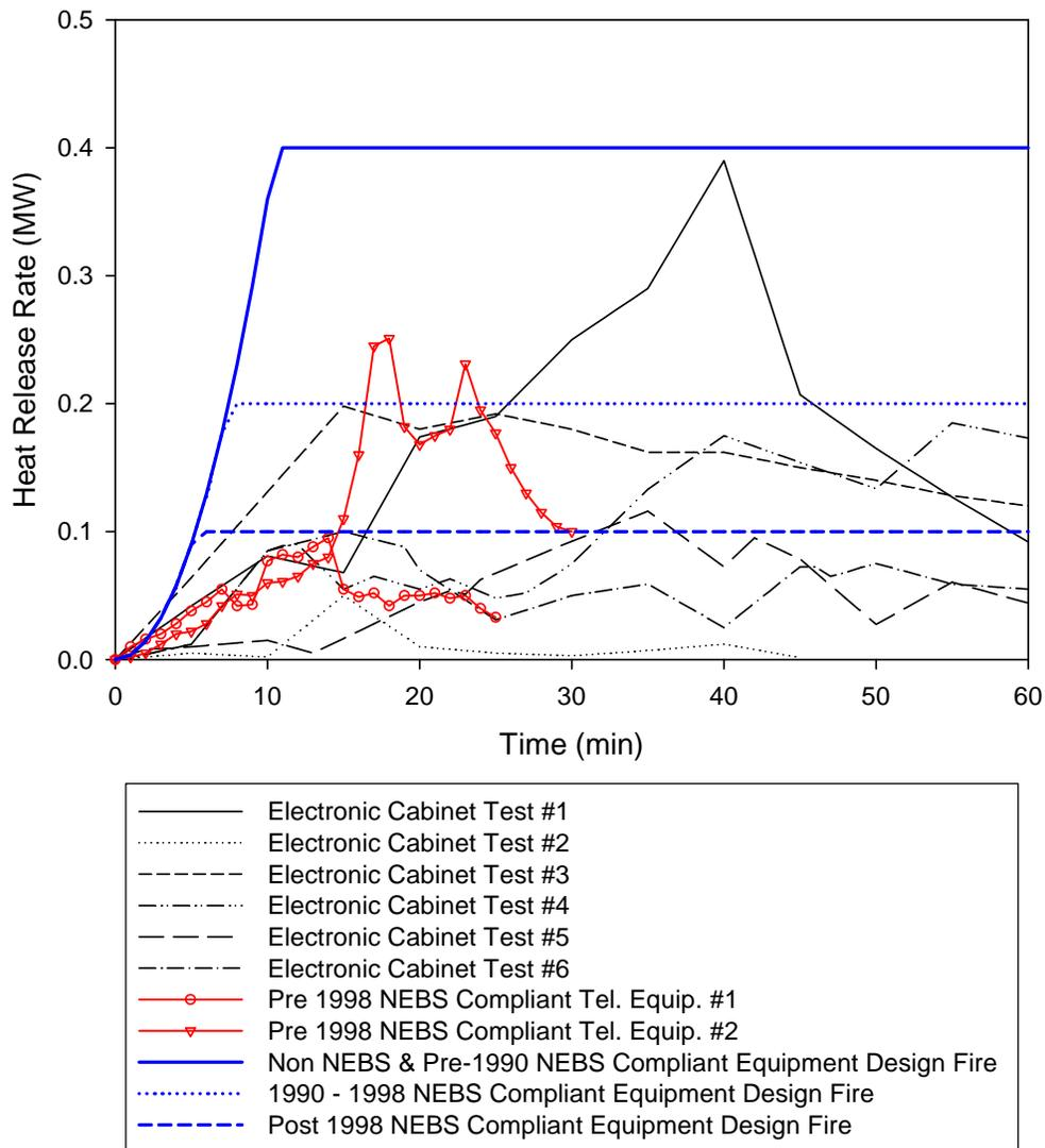
Figure 7 – Electronic Equipment Fire Tests & Design Fires
