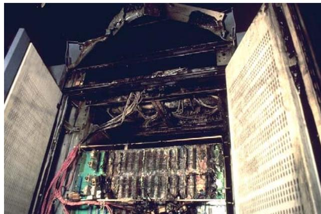
**Figure 6 – Results of NEBS Fire Test on 2002 vintage equipment**
