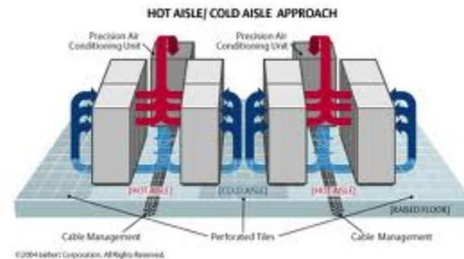
**Figure 2 – Typical hot/cold aisle cooling system**
