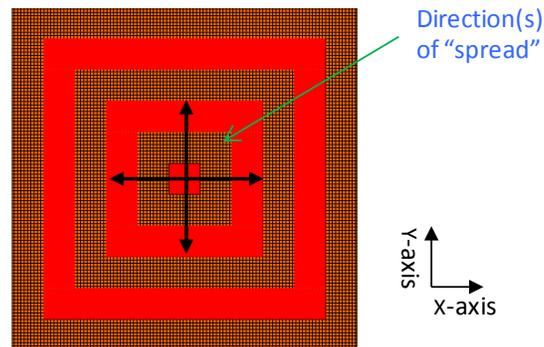
Figure 4 – Image Illustrating Lateral Fire Spread used in Fire Scenario 1
