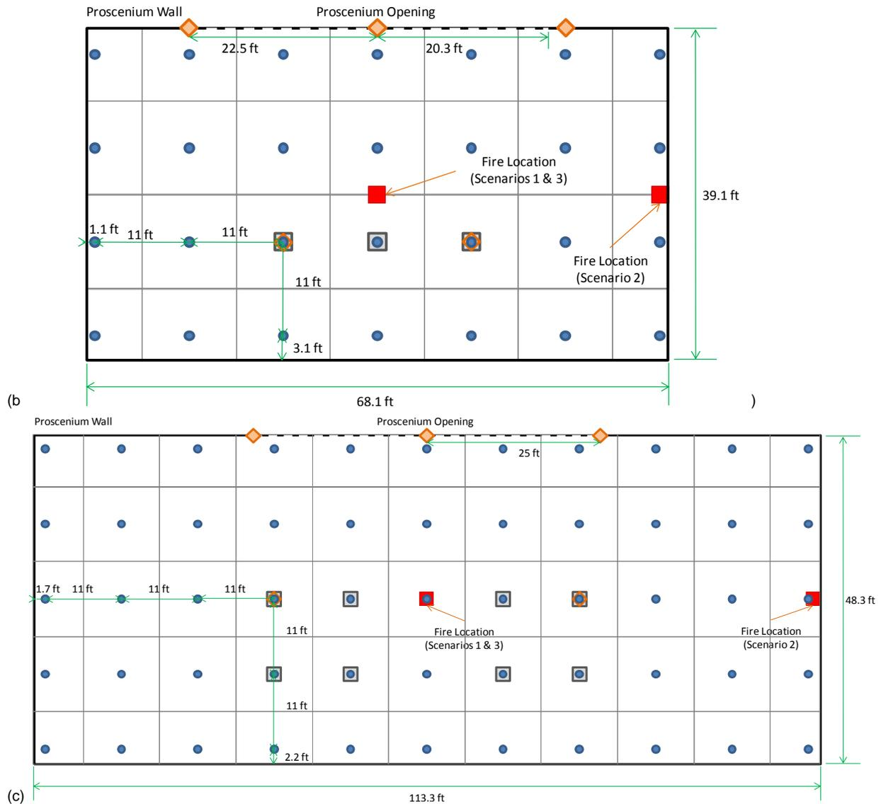
Figure 7 - Instrument layout shown in reflected-ceiling plan in the (a) small, (b) medium, and (c) large theatre models (● - sprinkler; ◆ - heat detector; □ - smoke vent fusible link; ■ - fire locations).
