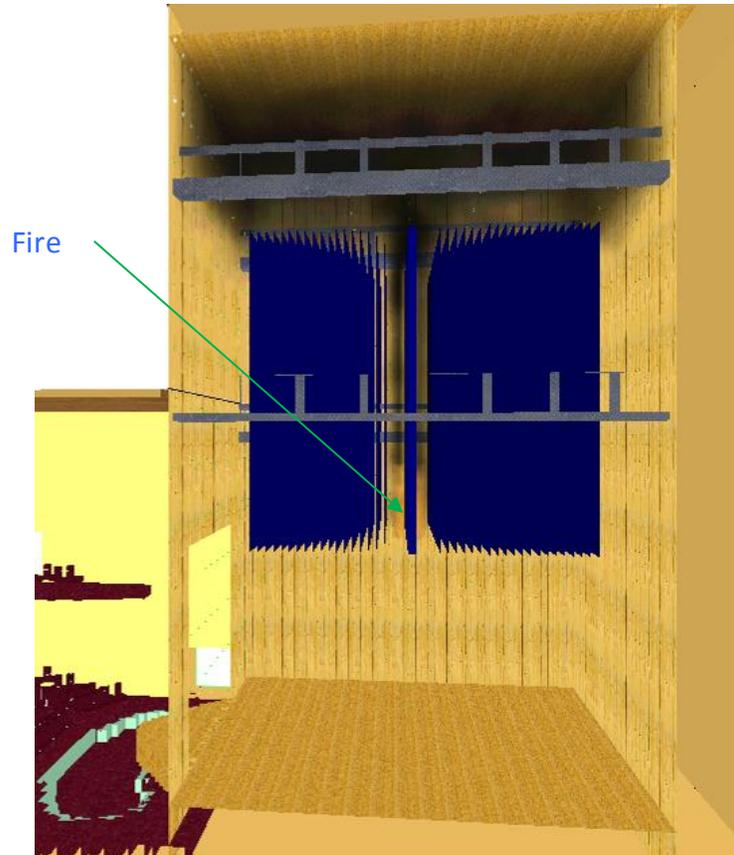
Figure 3 – FDS Image showing Location of the Fire in Fire Scenario 3 in the Medium-sized Theatre
