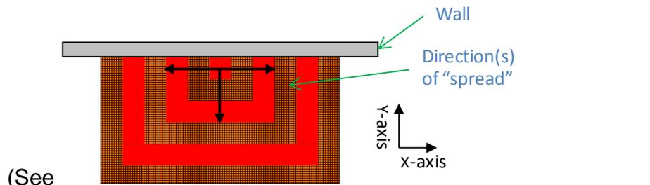
Figure 5 – Image Illustrating Lateral Fire Spread used in Fire Scenario 2.
