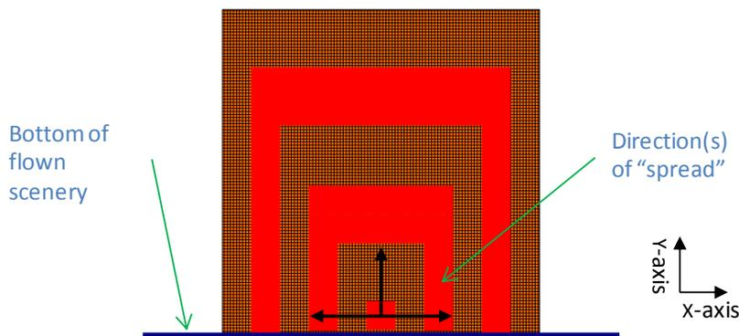
Figure 6 – Image Illustrating Vertical Fire Spread used in Fire Scenario 3
