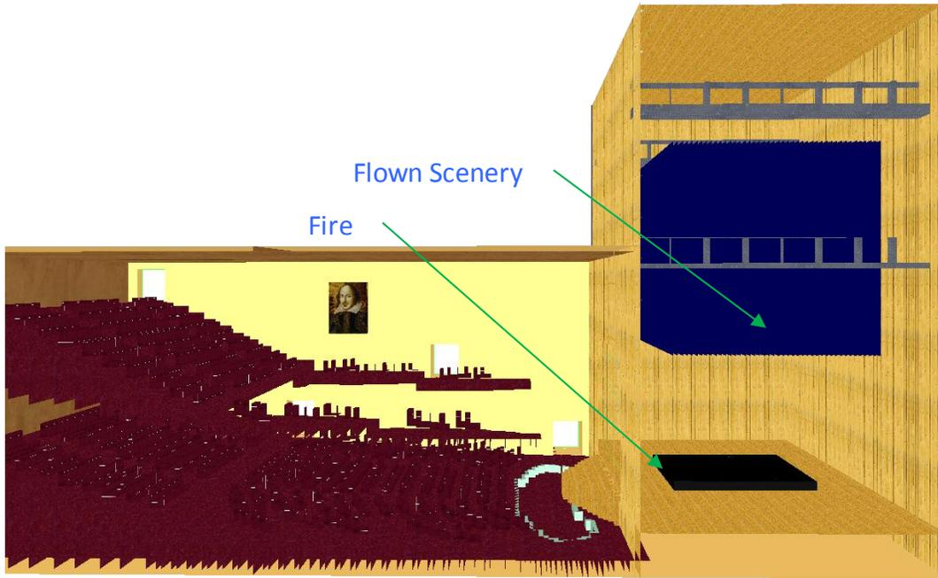
Figure 1 – FDS Image showing Location of the Fire in Fire Scenario 1 in the Medium-sized Theatre
