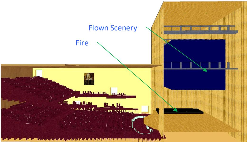
Figure 2 – FDS Image showing Location of the Fire in Fire Scenario 2 in the Medium-sized Theatre
