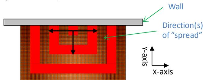
Figure 5 – Image Illustrating Lateral Fire Spread used in Fire Scenario 2.
