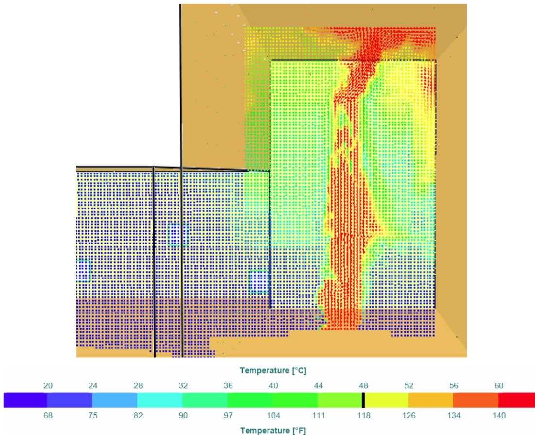
**Figure 9 – Velocity vectors colored by temperature shown on a contour section through the center of the stage in the medium-sized theatre for Scenario 1**
