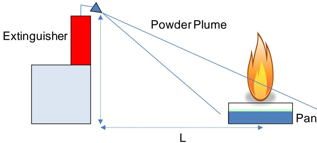
**Figure 1. Test Configuration for Class B fires**
