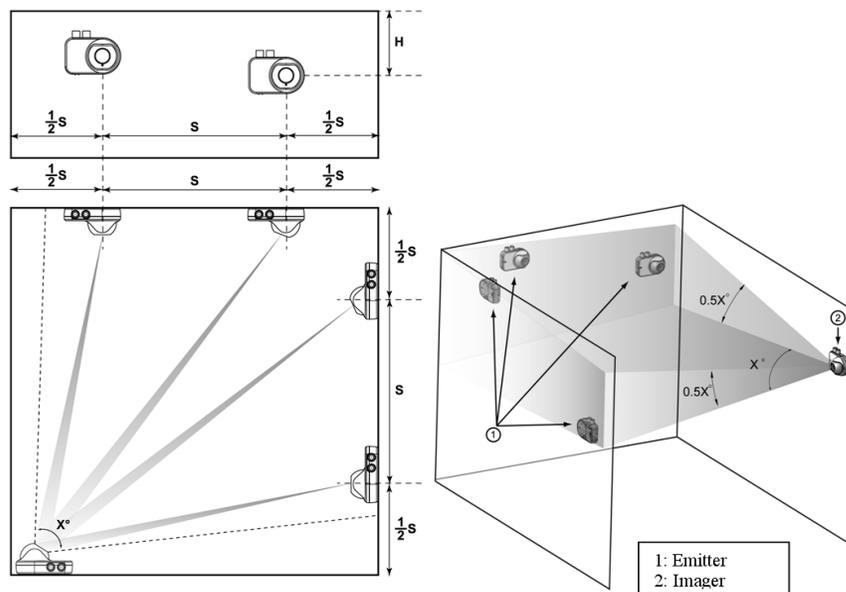
Figure 2 Multi-Emitter area OSID layout
