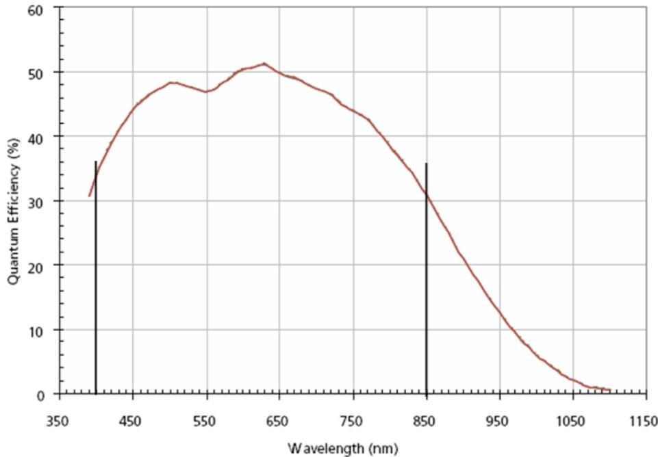
**Figure 5 - Imager Quantum Efficiency vs. Wavelength Curve**
