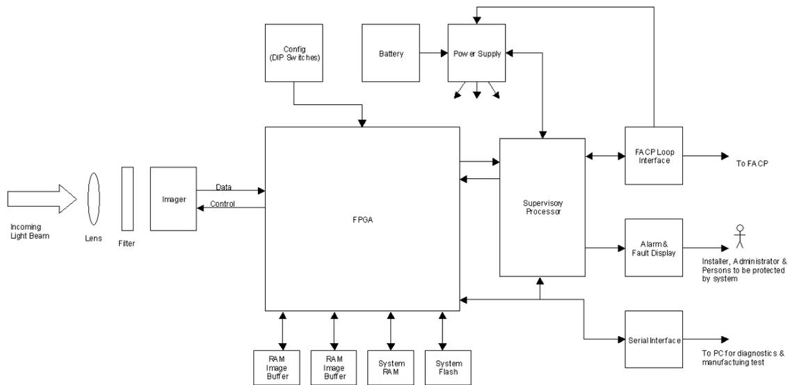
**Figure 4 Imaging Unit Physical Architecture**
