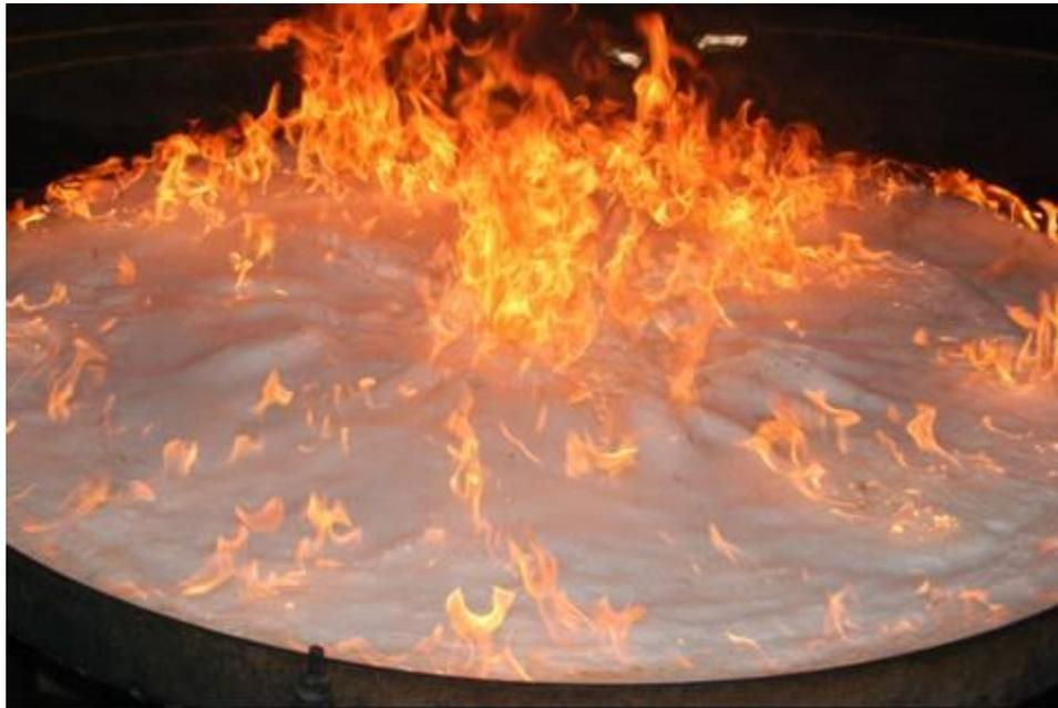
**Figure 1. Burn back test on gasoline, showing spread of flames over the foam-covered region.**
