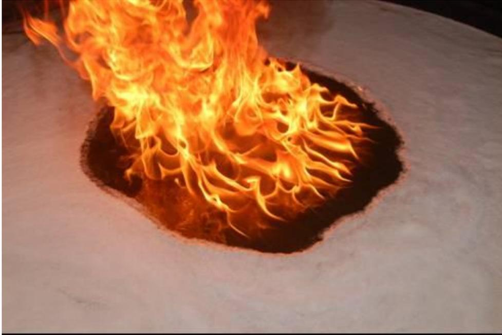
**Figure 4. Burn back test on biodiesel. Unlike the JP-5 burn back, in which the entire foam-free area is covered by flames, in this test there is a "standoff distance" between the flame and the edge of the foam-covered area.**
