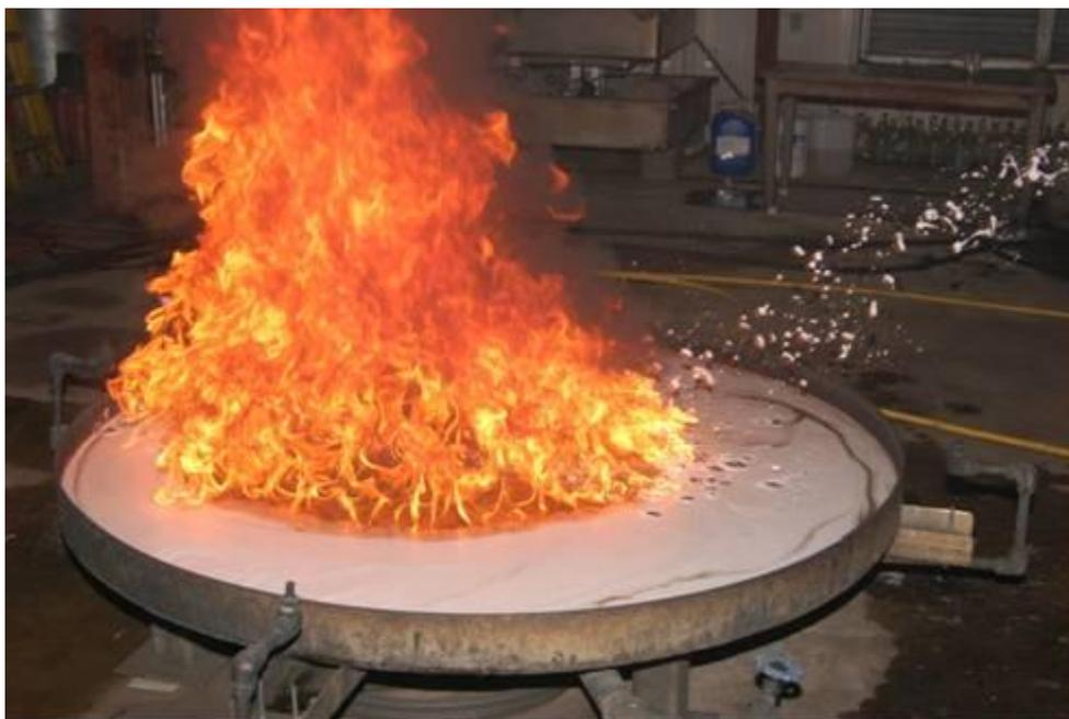
**Figure 3. End of burn back test with JP-5. Unlike the gasoline test, the fire is confined to a well-defined foam-free area of the fuel surface. The foam-covered region does not have flames isolated from the main fire.**
