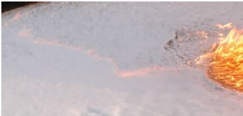
**Figure 2. Transient "ghost flame" sweeping across foam-covered surface in gasoline burn back test. Such flames occur periodically before sustained ignition**
