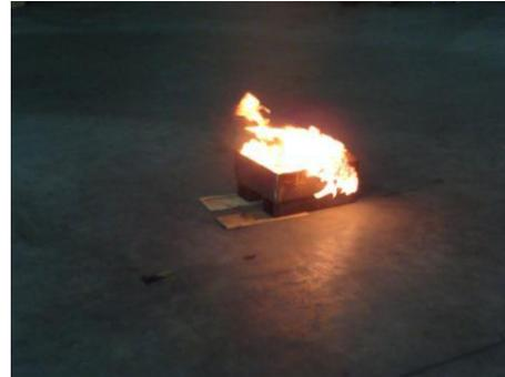
**Figure 11. A heptanes pan fire under wind conditions**
