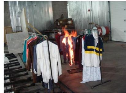
**Figure 17. A cloth fire located between two cloth racks**
