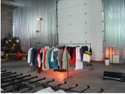
**Figure 15. A heptane fire located between two cloth racks**
