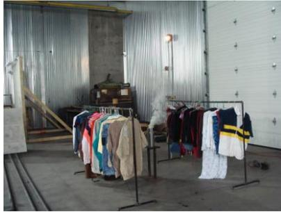
**Figure 16. A paper fire located between two cloth racks**
