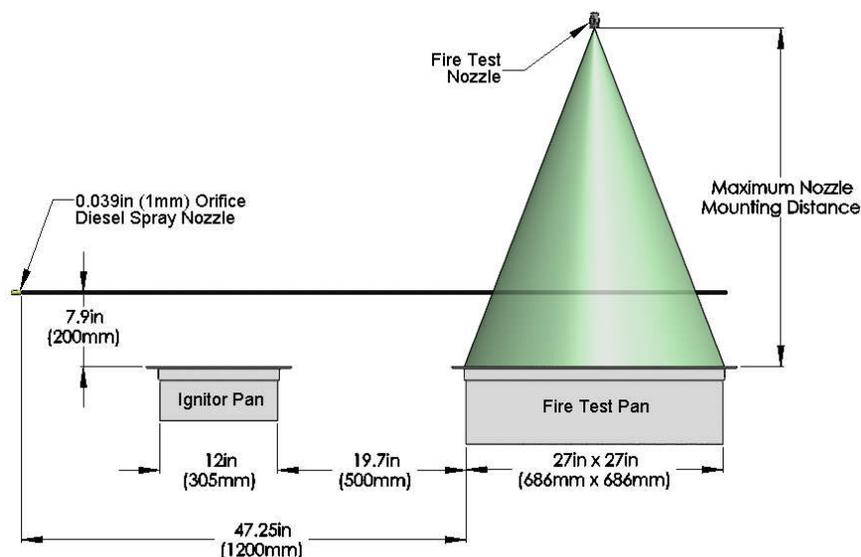
**Figure 4 Direct application fire test setup**
