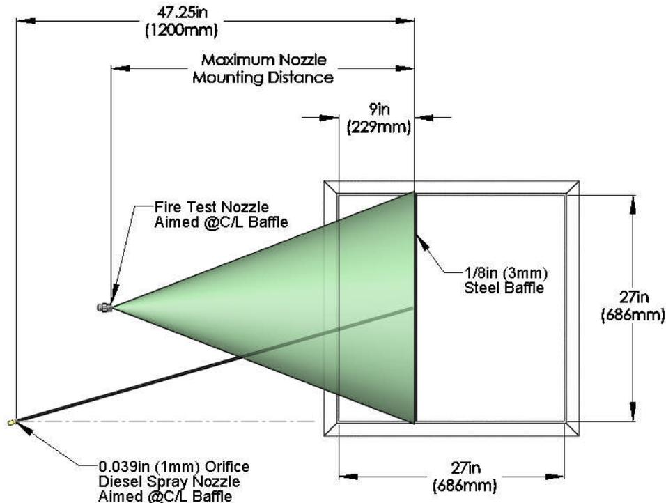
**Figure 6 In-direct application fire test with baffle (top view)**
