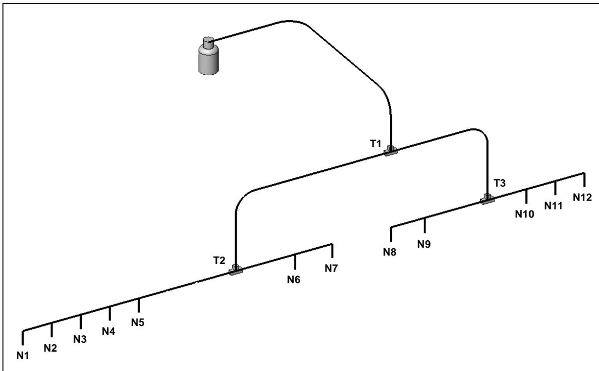
Figure 3 Typical hose distribution network
