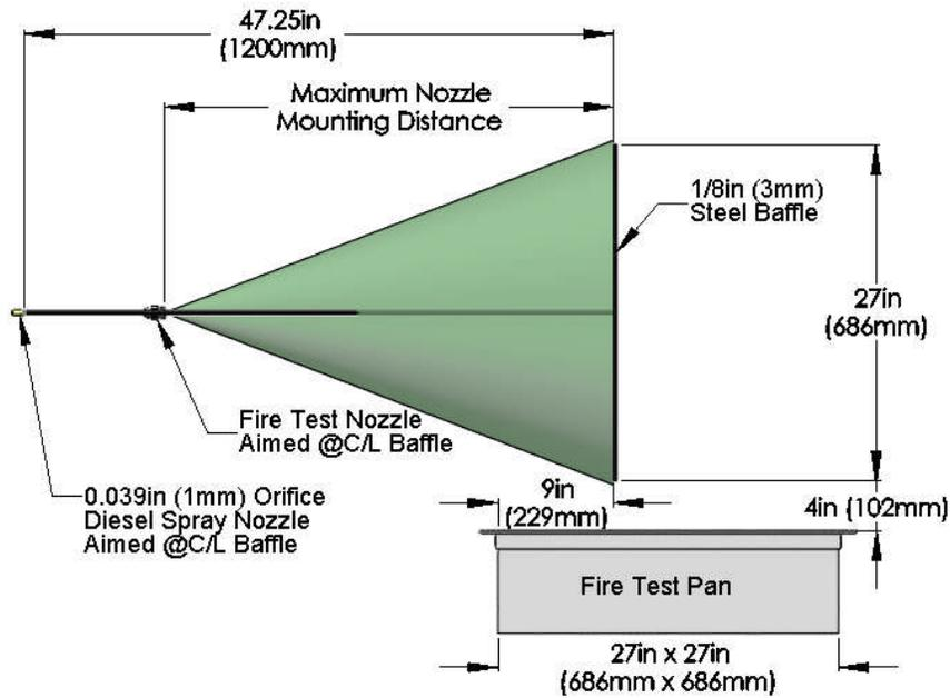
**Figure 5 In-direct application fire test with baffle (side view)**
