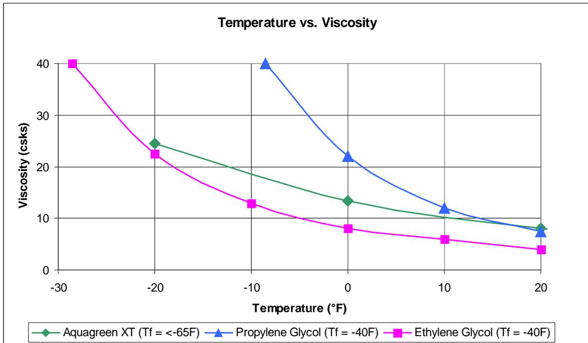
Figure 1 Viscosity data for various freeze-protected solutions
