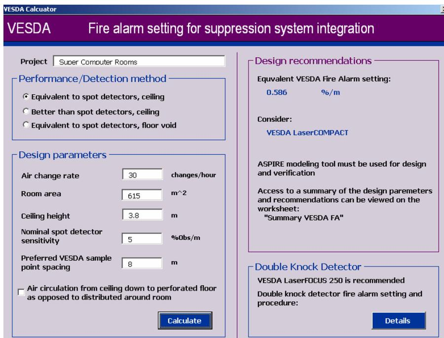
Figure 7: Application Tool: ASD **Fire** alarm setting for gaseous suppression activation
