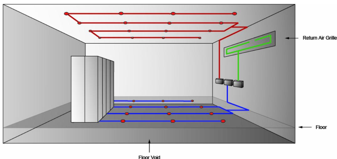
For ASD detector, average transport time was used. For spot-type detectors, the detector activation relies on number of factors including temperature raise, air velocity and smoke density [17]. To simplify the analysis, 20 seconds entry lag time were adopted as a conservative approximation to the spot-type detectors after the smoke density has reached the detector nominal sensitivity.
