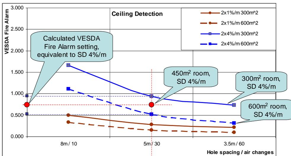
3. Calculate improved ASD detector **Fire** alarm setting, taking into account number of factors such as ceiling height, airflow, actual sampling point spacing applied.
