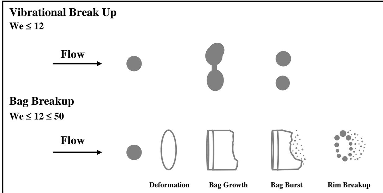
**Figure 9:** Breakup mechanisms
