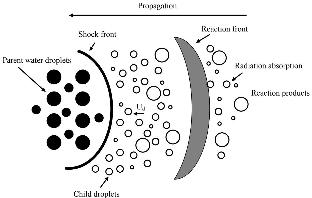
**Figure 1:** Interaction of water droplets in detonation process
