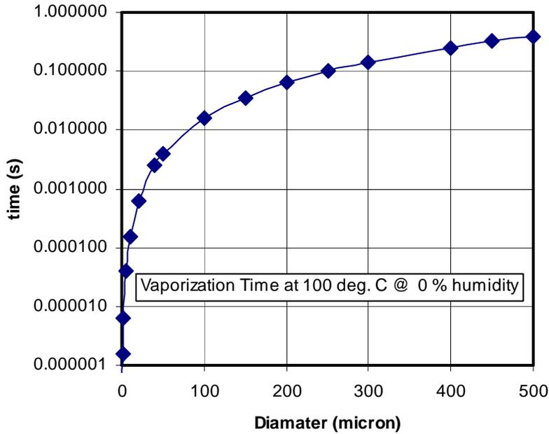
**Figure 10:**  $d^2$ -law evaporation time scales of child droplets from the shock-induced droplet breakup process
