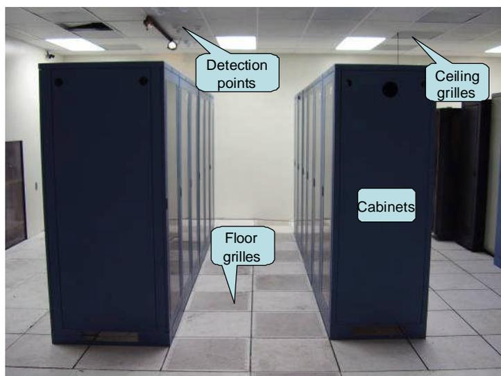
**Figure 1** Datacom Facility Mock-up (In-situ Testing)
