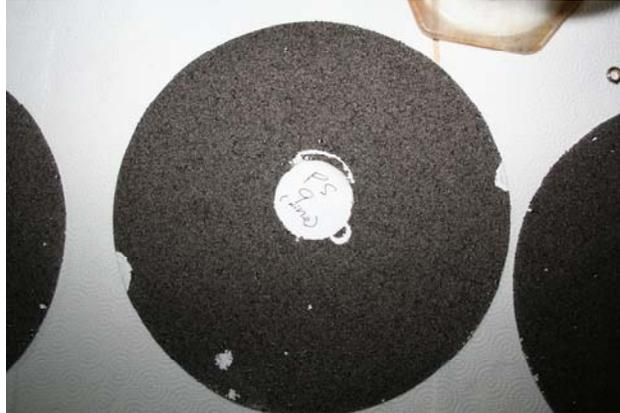
Fig 13. Photo of the polystyrene smoke particles deposited on a filter paper.
