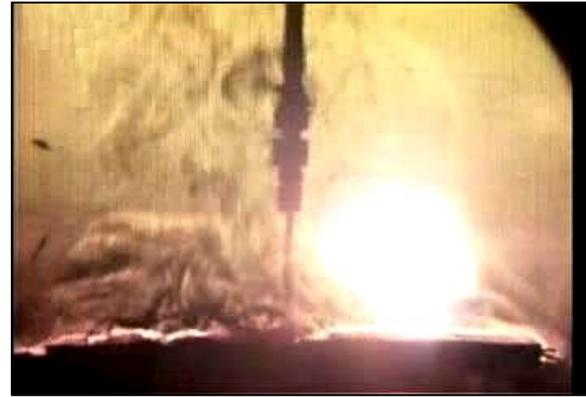
**(ii) Ignition of fuel on the surface of the hot plate**
