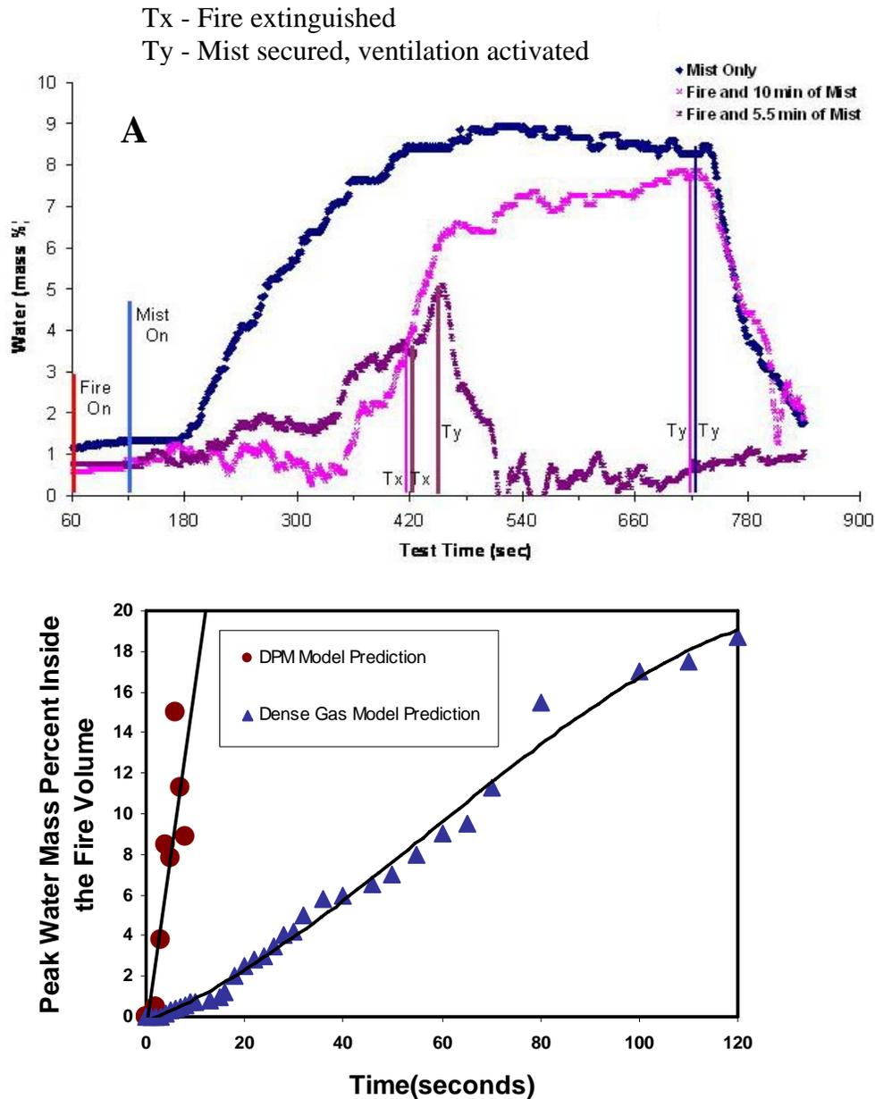
Figure 1: Comparison of A) measured water concentration history near the firebase and B) DPM and Dense Gas Model predictions in compartment fire tests. 1B computation times 0 – 120 sec correspond to 1A test times of 120 – 240 seconds.
