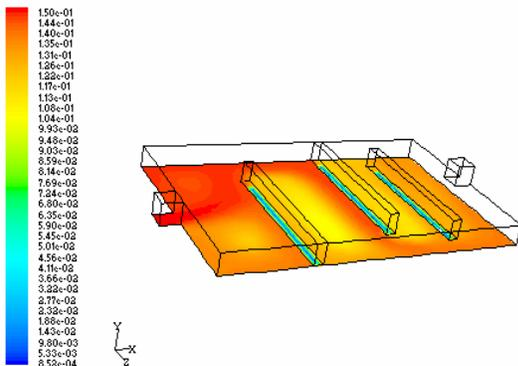
Figure 8A: Dense gas model mass fraction contours
