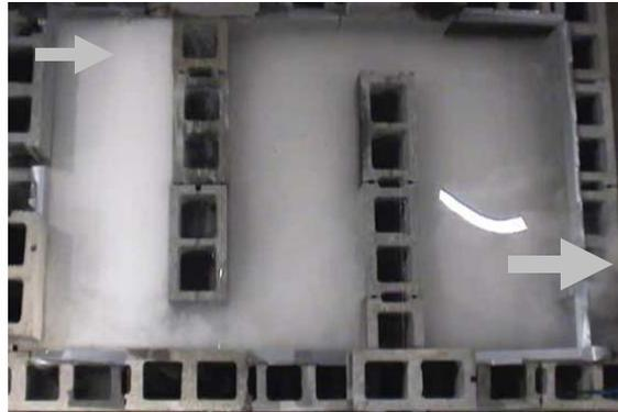
Figure 8B: Ultra fine mist flow experiment in a flow channel
