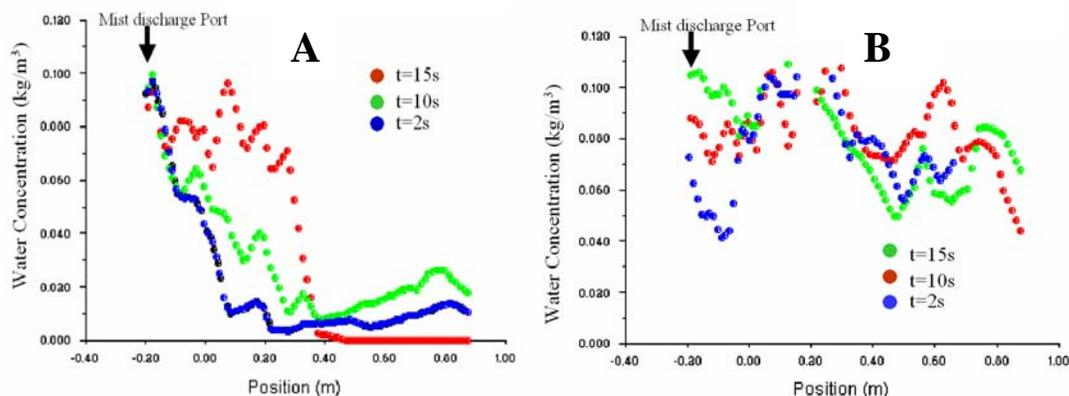
Figure 6: DPM centerline concentration of mist at various time steps for: A) a low discharge velocity of 1.0 m/s, and 2) a high discharge velocity of 5 m/s.
