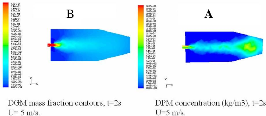
Figure 3: Predicted water concentration by: A) Dense Gas Model (DGM) and B) DPM at  $t=2 \text{ s}$  using discharge velocity  $5.0 \text{ m/s}$
