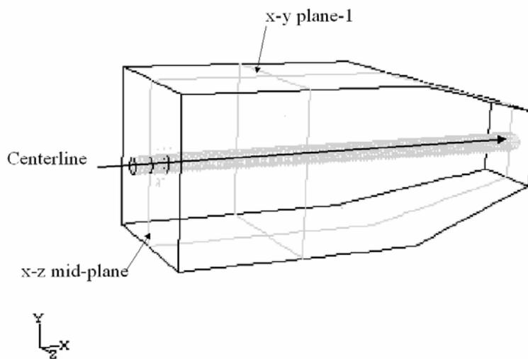
Figure 2: Geometry of flow channel used for simulating ultra fine mist flow
