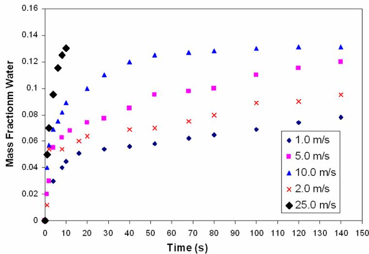
Figure 5: Time-dependent water mass fraction maximum at x-y plane-1 normal to flow -DGM Model
