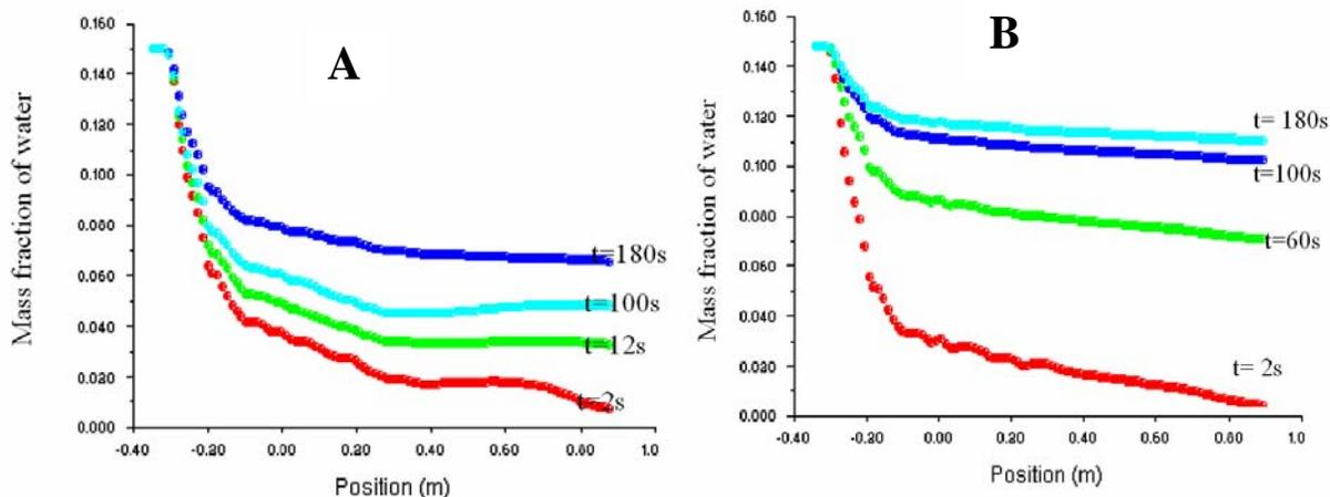
Figure 4: DGM centerline concentration of mist at various time steps for: A) a low discharge velocity of  $1.0 \text{ m/s}$ , and 2) a high discharge velocity of  $25 \text{ m/s}$ .
