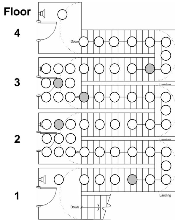
**Figure 5: Stairwell intelligibility was measured at numerous locations (circles), with five to ten readings at most locations and 100 measurements taken at the shaded circles. The landings to the right are reversed for this representation.**
