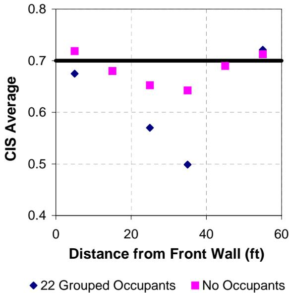
**Figure 3: Intelligibility measurements in a classroom with and without occupants. The occupants were seated near the center of the room, and four speakers were sounding, one in each corner of the room. No measurements were taken 4.5 m (15') or 13.6 m (45') from the front wall**
