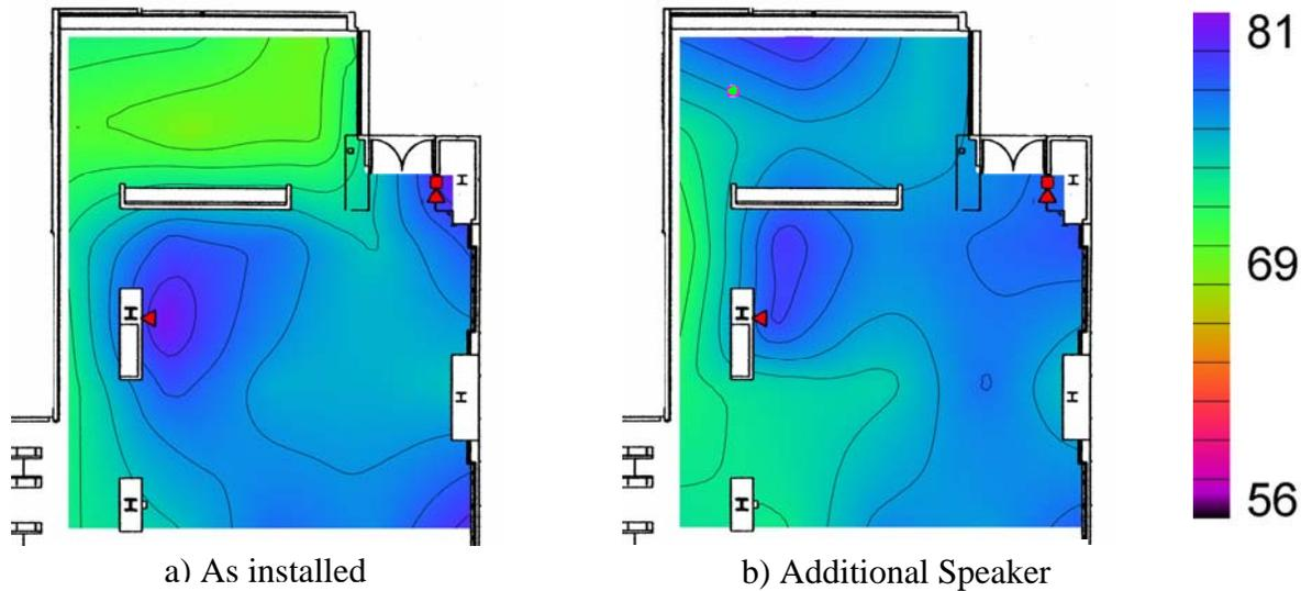
**Figure 1: Intelligibility measurements (shown in CIS\*100) for the dining area of a cafeteria in a commercial building. a) shows the results for the system as installed, while b) illustrates the impact of an additional speaker. This dining area consists of a dining alcove (the small area in green at the top of a) and a main dining area. Only half of the entire space is shown.**
