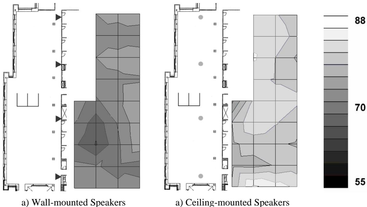
**Figure 2: Intelligibility measurements for an office area with an open floor plan are shown. a) and b) provide plan views of the office space (left), including locations of speakers (triangles and circles, respectively), and a contour map of the CIS measurements (right) for wall- and ceiling-mounted speakers, respectively. The figure illustrates the improvement of intelligibility possible through relocation of speakers.**
