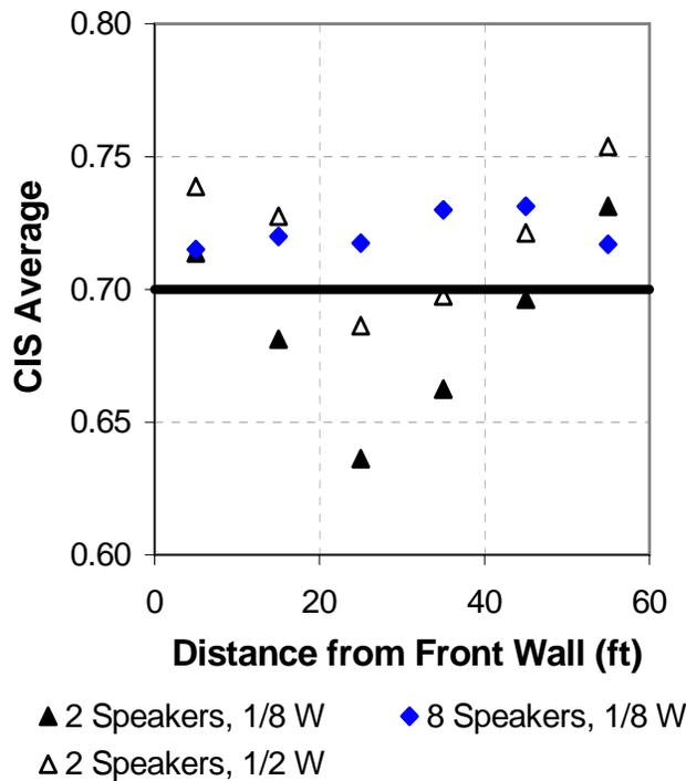
**Figure 4: Intelligibility measurements in a classroom with different numbers of speakers sounding, showing the influence of measurement location and supplied energy on intelligibility**
