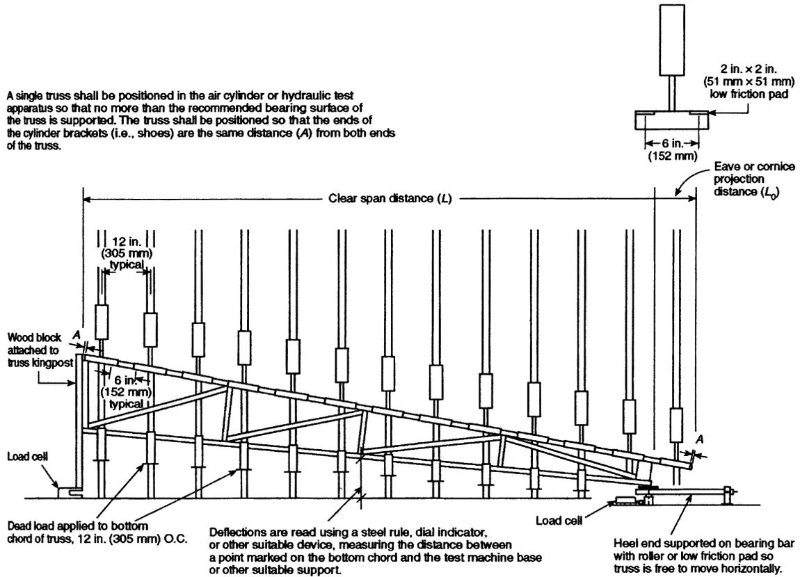
(2) When tested in groups of two or more, the top chords are permitted to be sheathed with nominal 1/4-inch x 12-inch plywood strips. The plywood strips shall be at least long enough to cover the top chords of the trusses at the designated design truss spacing. Adjacent plywood strips shall be
