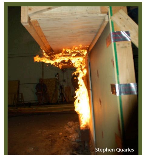
Lateral flame spread was reduced when a combustibile soffit material ignited in this test of a soffited-eave with a combustibile soffit material.
