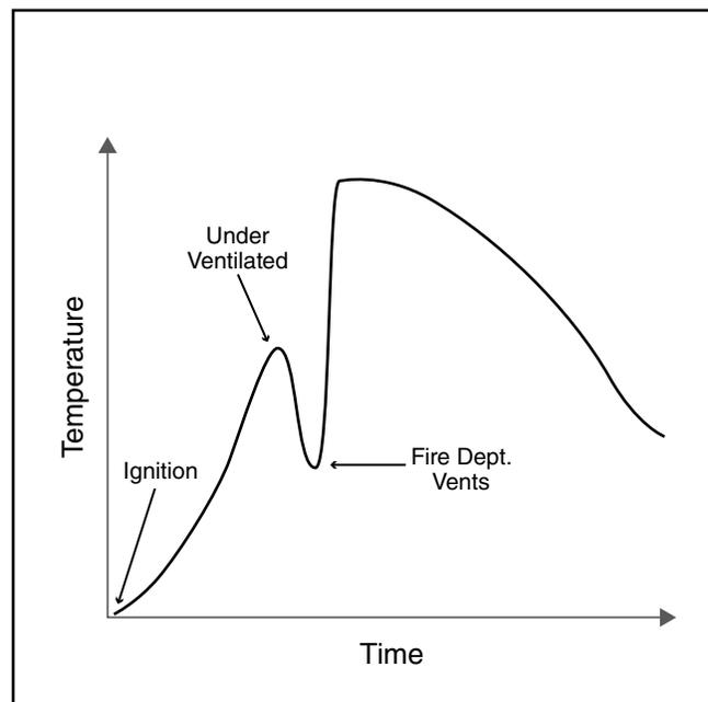
**Figure 5** shows the temperature in the living room during the experiment described in the previous paragraph. Notice the shape of the temperature curves with respect to time: fire growth, followed by decay, or a decrease in heat-release rate, which is then followed by a significant and rapid increase in heat-release rate and gas temperature because of the increased availability of oxygen to the fuel-rich environment of the fire room.
