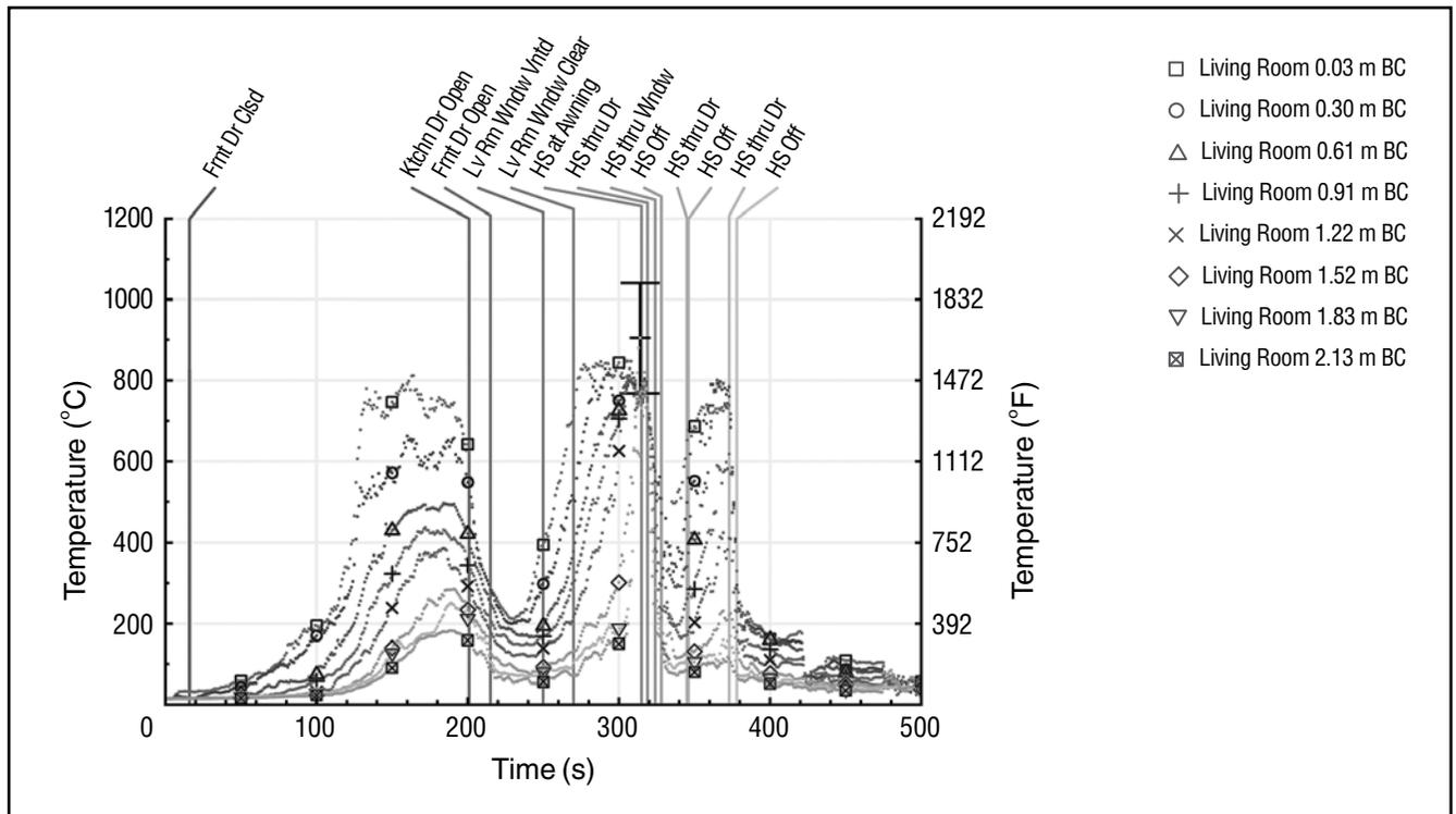
**Figure 6: Temperature time-history curves comparing the temperature of the fire-compartment (lower) side of oriented strand board (OSB) subflooring and the temperature of the upper-level room side of the OSB. The measurement locations are separated only by the OSB, which is approximately 18 mm (0.75 in) thick.**
