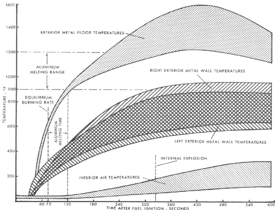
**Figure 9—Summary of the Time-Temperature Data Obtained for the Aircraft Loading Walkway during Fire Exposure [Geyer, 1973]**
