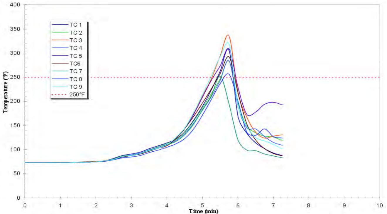
**Figure 11—Thermocouple Temperatures during Fire Exposure Test [Luna, 2005]**
