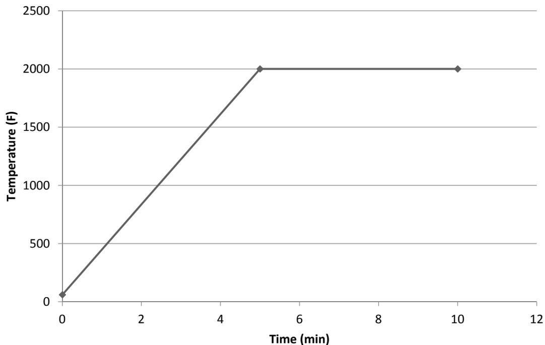
Figure 10—UL 1709 hydrocarbon fuel fire threat [UL, 2011]
