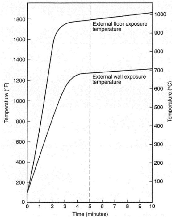
**Figure 8—Time-Temperature Curves for Fire Testing of Aircraft Loading Walkways [NFPA, 2013]**
