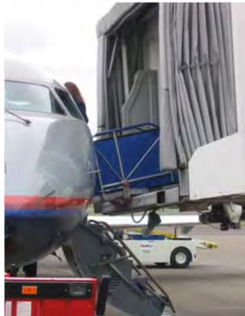
**Figure 20—Example loading walkway adapter**
