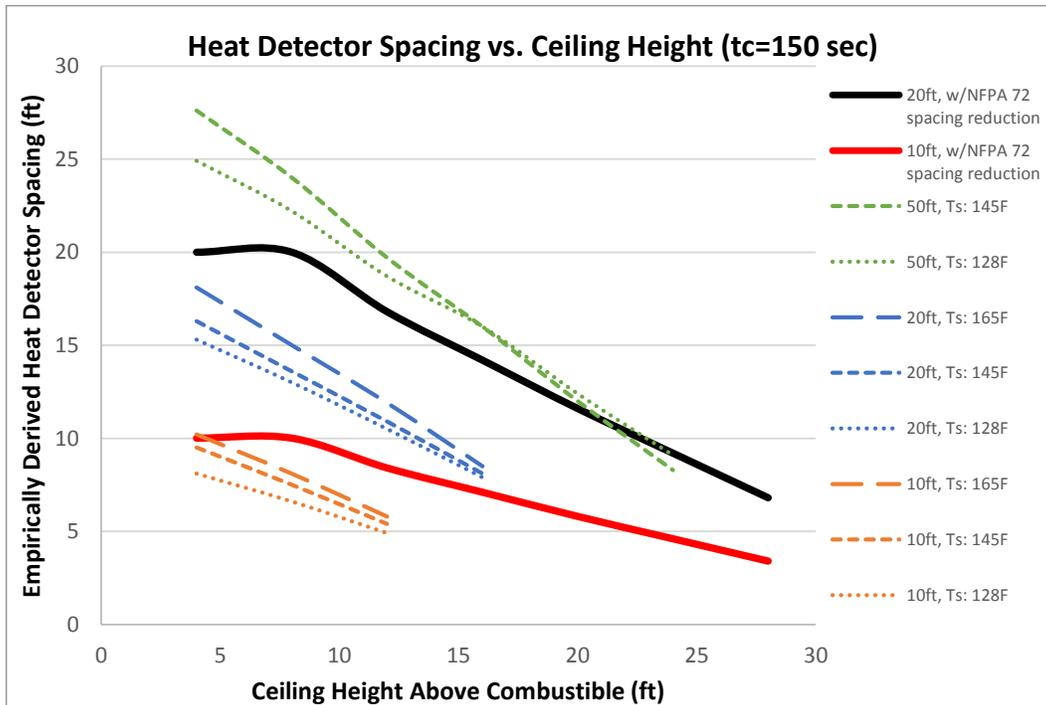
Figure 3: Comparison of the ceiling height above combustibles as required in NFPA 72 and in the Heskestad and Delichatsios paper for a critical time of 150 seconds. [3] [5]
