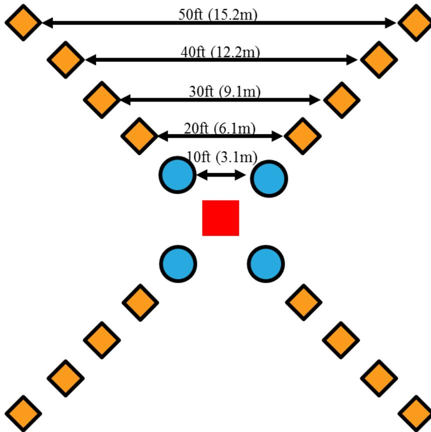
Figure 1: Heat Detector testing arrangement. The blue circles represent sprinklers whereas the orange diamonds represent the heat detectors. An 1138 BTU/sec (1,200 kW) ethanol/methanol fire is ignited. The greatest detector spacing that produces an alarm before a sprinkler actuates is the listed spacing for the detector. [1]
