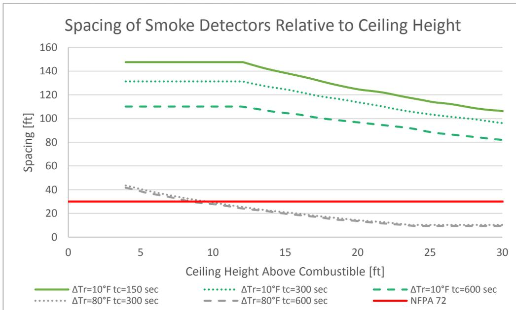
Figure 4: Smoke detector spacing v. ceiling height for temperature rise at response and critical fire times. The different colors indicate different temperature rise characteristics and the different curves represent different critical times (i.e. growth rates with  $t_c = 150, 300, 600$ ) [3]. For reference the spacing currently codified in NFPA 72 is indicated by a red line. [5]
