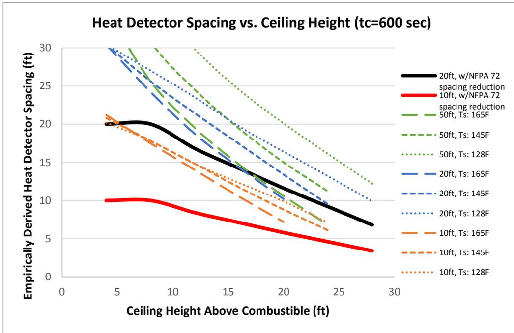
Figure 2: Comparison of the ceiling height above combustibles as required in NFPA 72 and in the Heskestad and Delichatsios paper for a critical time of 600 seconds. [3] [5]
