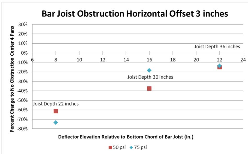
**Figure 4. Bar Joist Obstruction with Offset of 3 inches**
