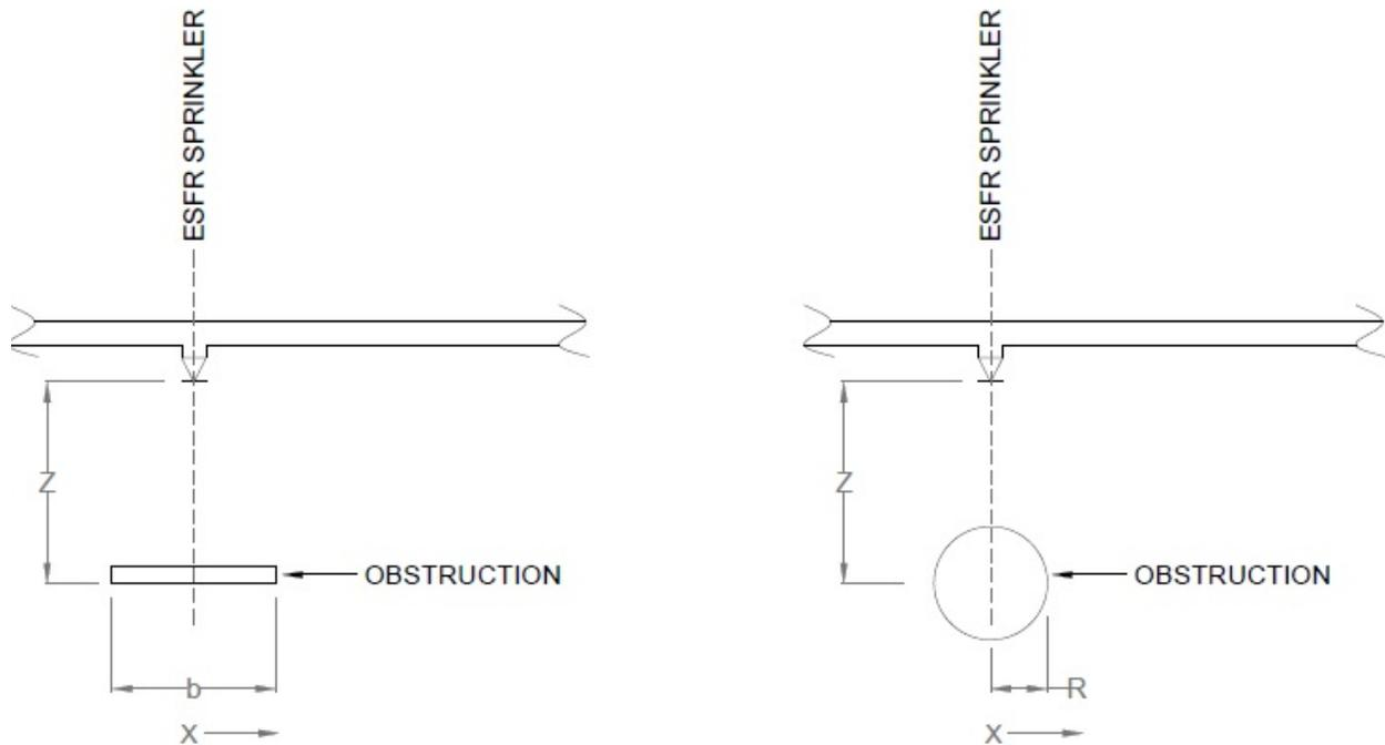
**Figure 6. Concept ADD Assembly for Miscellaneous Obstructions**
