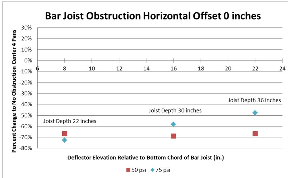
**Figure 3. Bar Joist Obstruction with Offset of 0 inches**
