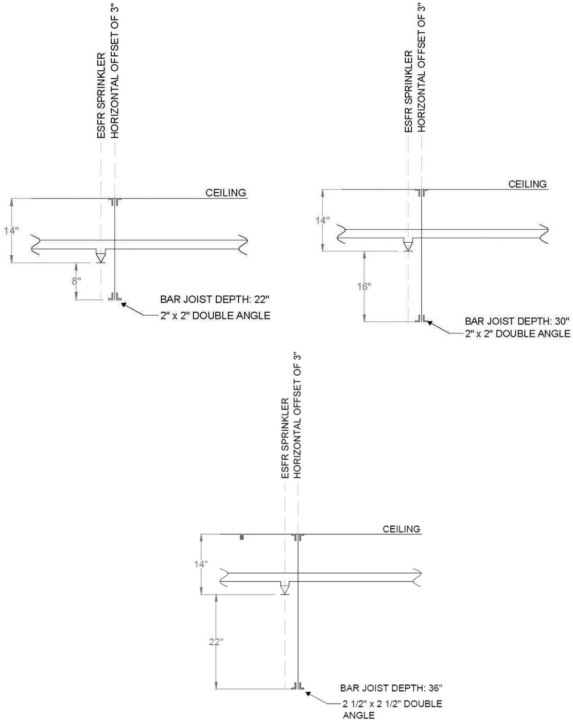
**Figures 1A-C. ADD Obstruction Assembly for Bar Joist Depths of 22, 30, and 36 inches and a Horizontal Offset of 3 inches**
