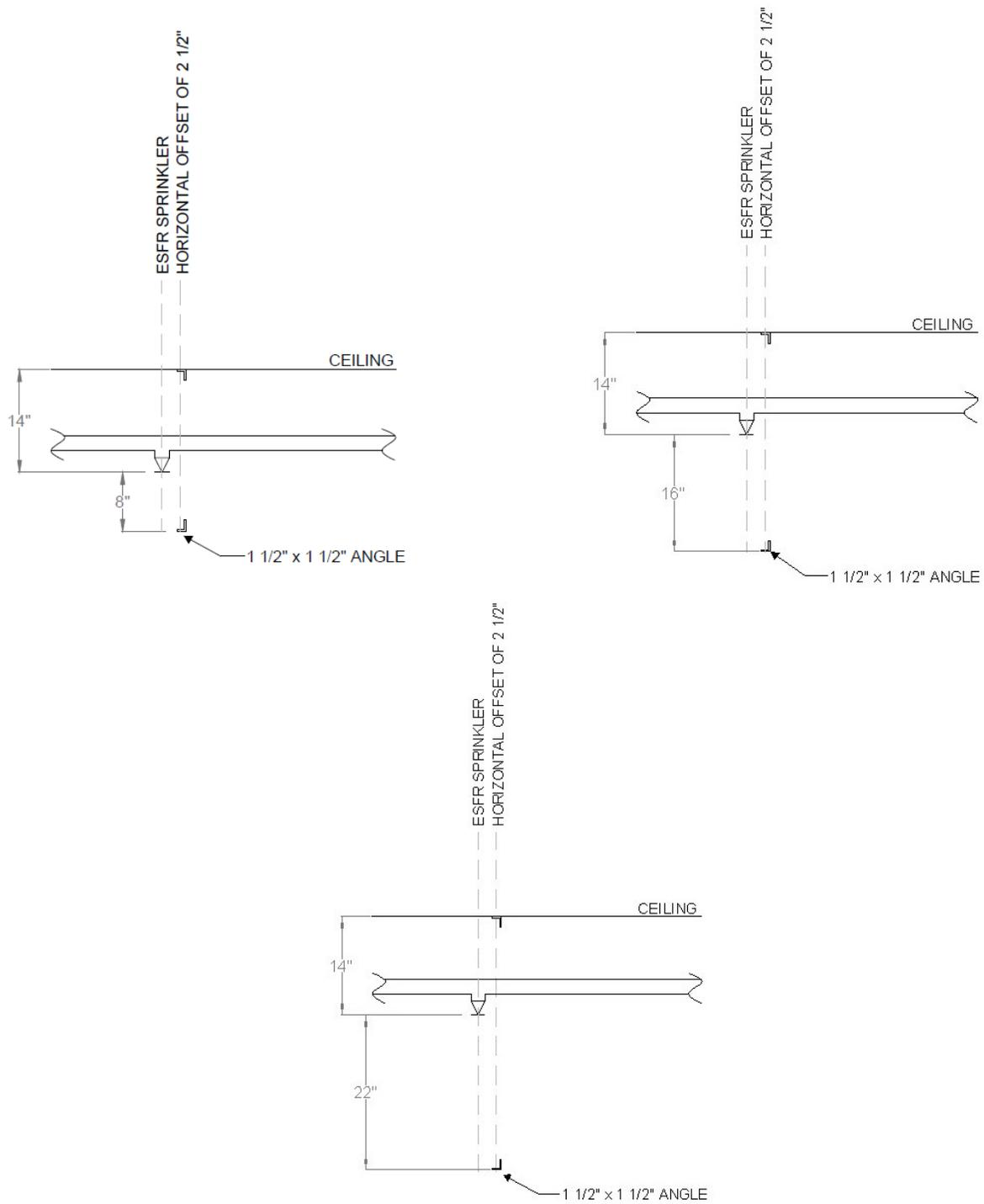
**Figures 2A-C. ADD Obstruction Assembly for Bridging Member With Horizontal Offset of 2½ inches**
