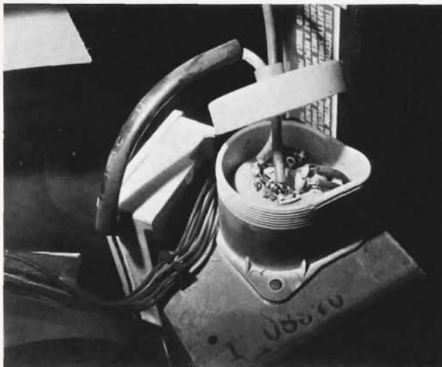
Photo 2. Polypropylene insulating cup and polyethylene cap surrounding base of high voltage tube.
