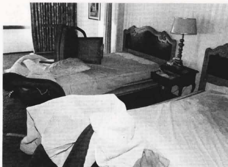
Two victims were found near the windows in this twenty-first floor room that was adjacent to the elevator lobbies. Note light smoke deposits on beds where pillows and bedding were removed. NFPA
