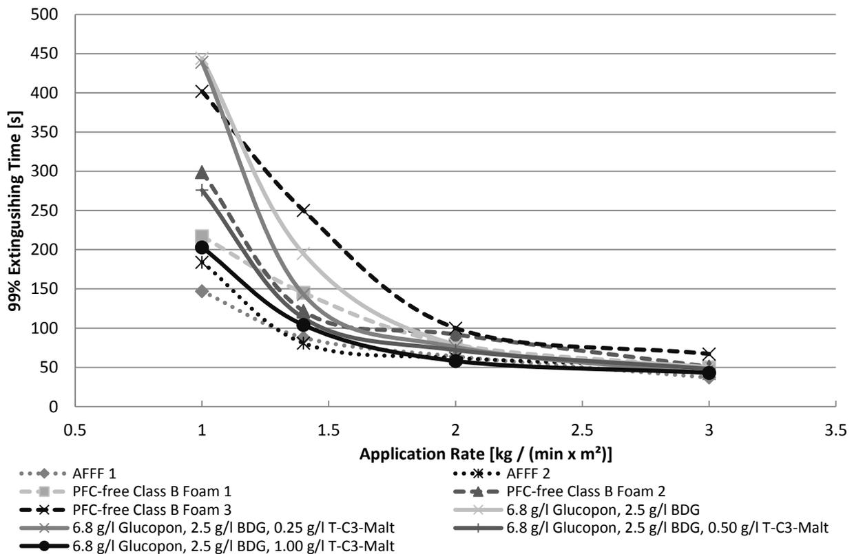
**Figure 2: Comparison of the 99%-extinguishing times of siloxane surfactant solutions and commercial firefighting foams.**
