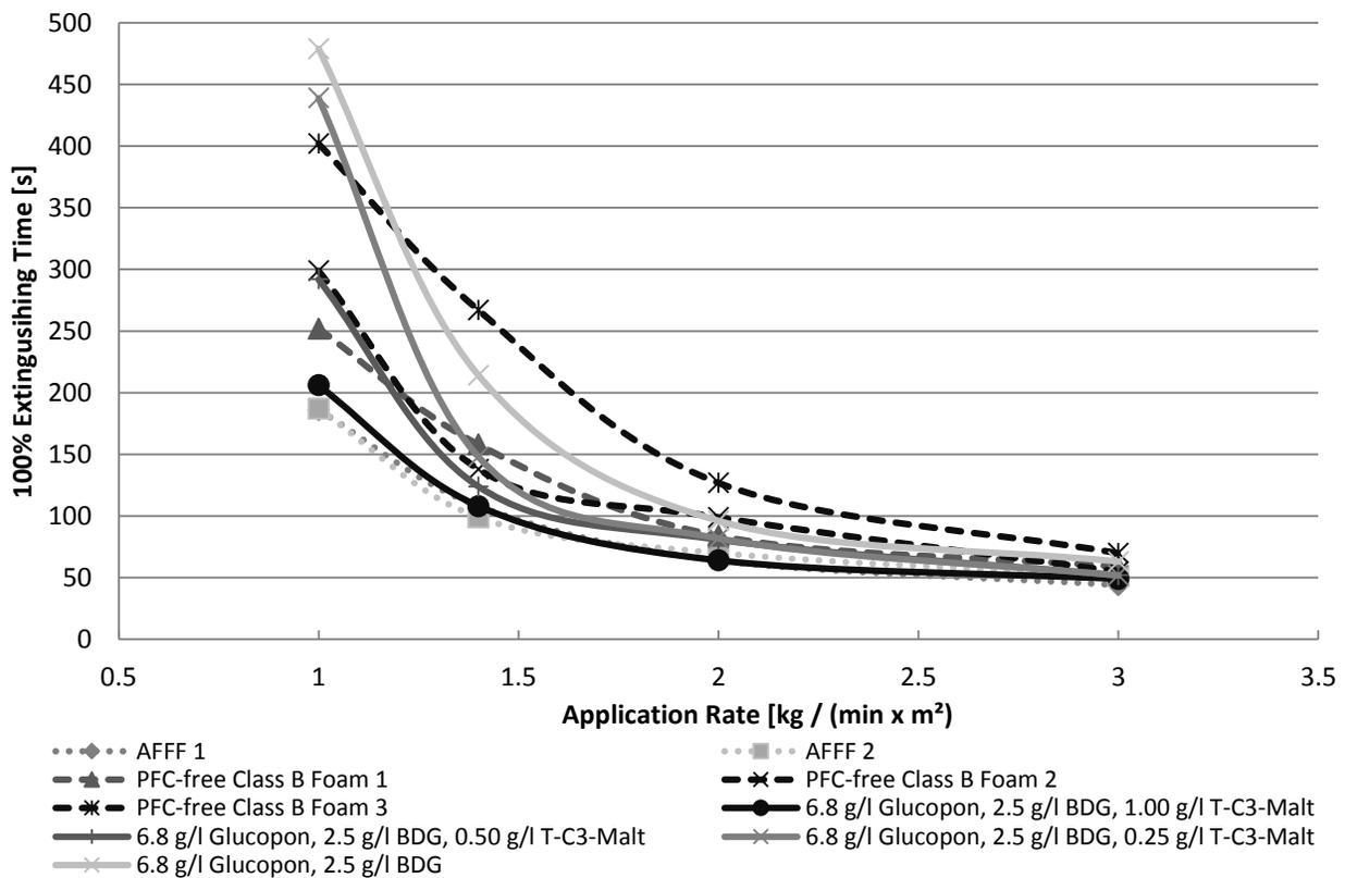
**Figure 3: Comparison of the 100%-extinguishing times of the surfactant solutions and various firefighting foams.**
