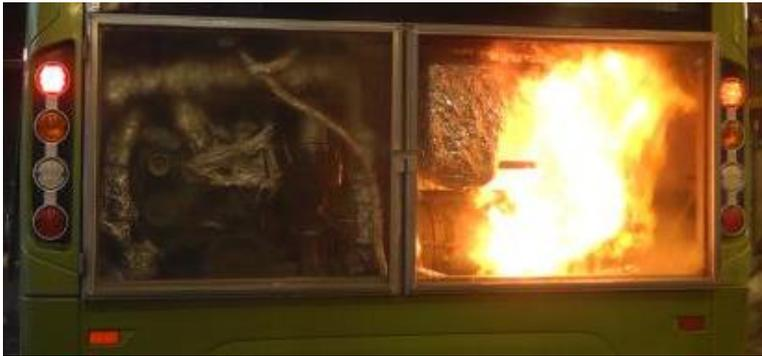
Fig. 5 Fast developing fuel spray fire
