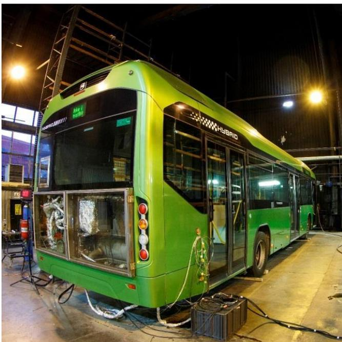
Fig. 4 City bus prepared for performing fire detection tests
