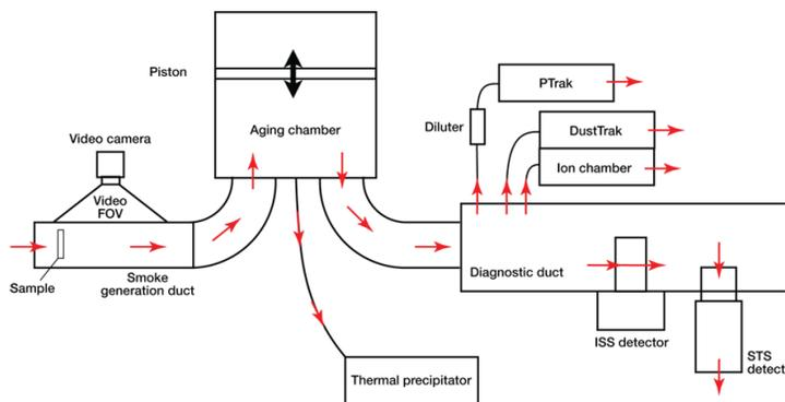
**Figure 1.** Schematic of the SAME hardware.
