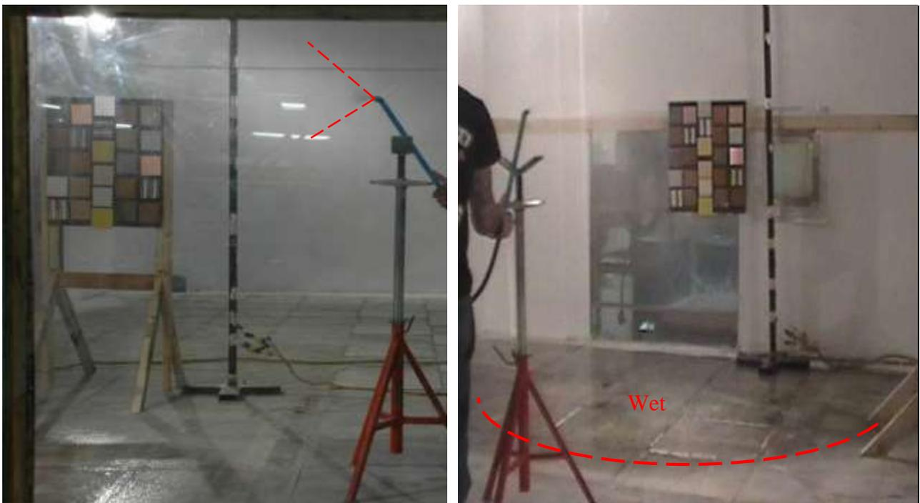
**Figure 5 – Typical water mist extinguisher spray pattern (left) and water deposited on the floor (right).**
