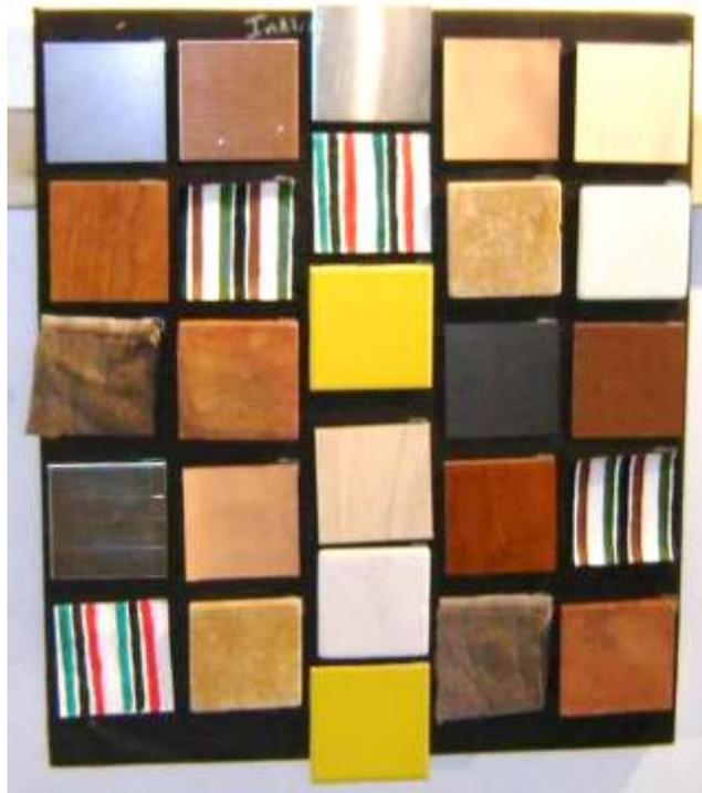
**Figure 1 – Typical sample array for exposure tests.**
