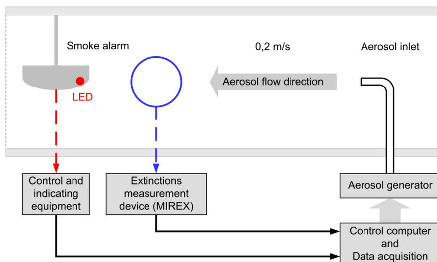
Figure 1 Principle of the measurement system
