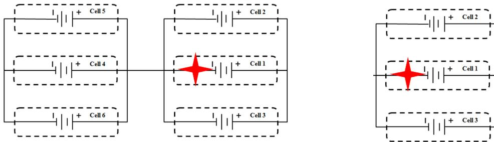
**Figure 1: 3P2S Battery Pack Configuration (left) and 3P configuration (right)**
