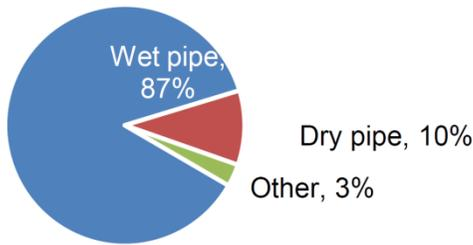
Fig. 1. Types of sprinklers found in U.S. structure fires: 2010-2014.
