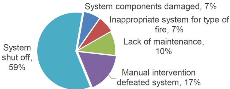
Fig. 5. Reasons for sprinkler failures: 2010-2014.
