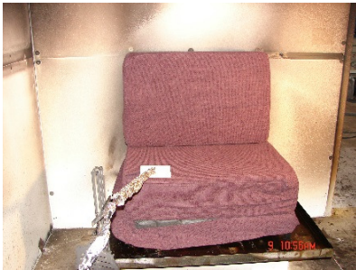
Figure 1. Chair mockup consisting of polyurethane foam slabs with cotton seat cushion and chair back cushion covers.
