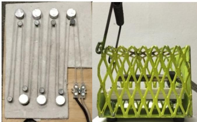
Fig. 1. BS 6266 Wire cradle (left) and Compact Incipient Smoke Detector Test Apparatus (CISTA) (right).
