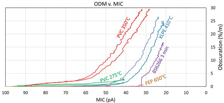
Fig. 3. Obscuration v. Ionization for wire sources in the smoke box.
