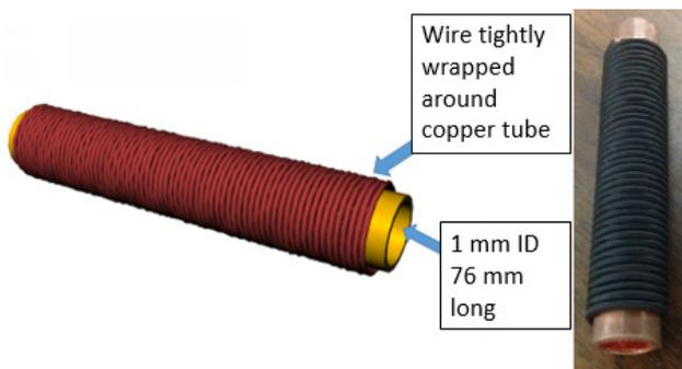
Fig. 2. Disposable wire cartridge used for CISTA smoke production.
