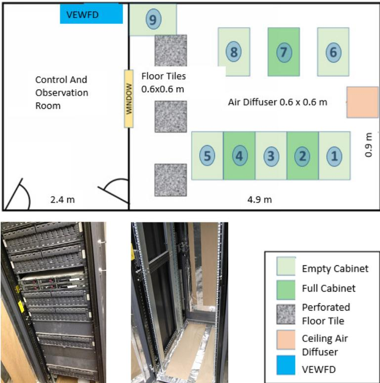
Fig. 5. Mock electrical cabinet test space and full (left) and empty (right) cabinets.
