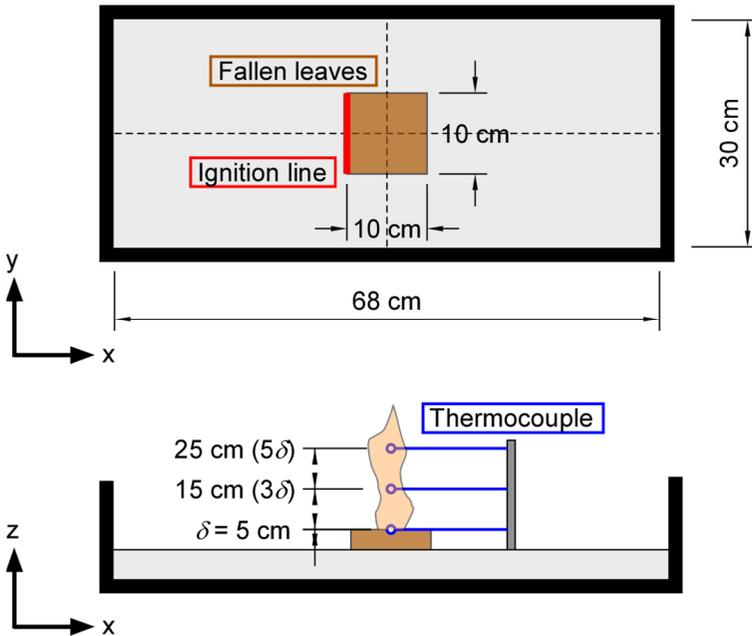
Figure 2. Setup of combustion experiment.
