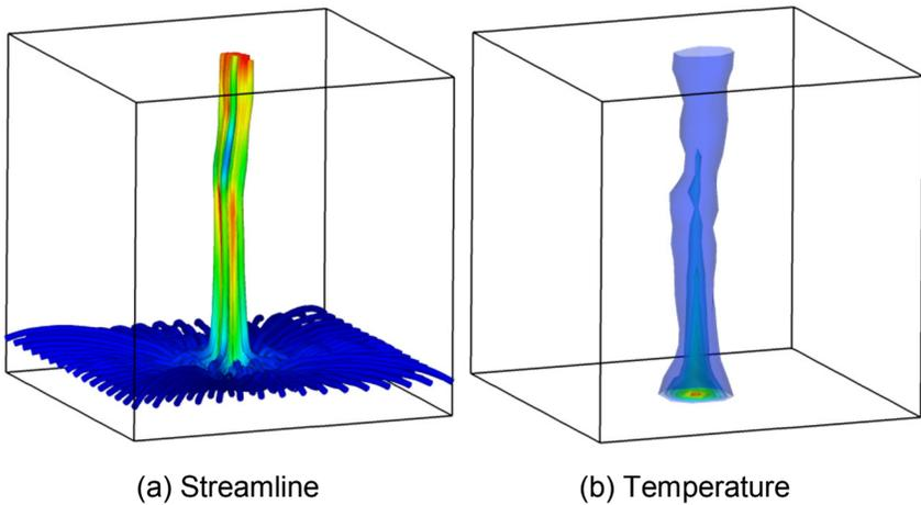
Figure 6. Numerical result of airflow around burning wood elements.
