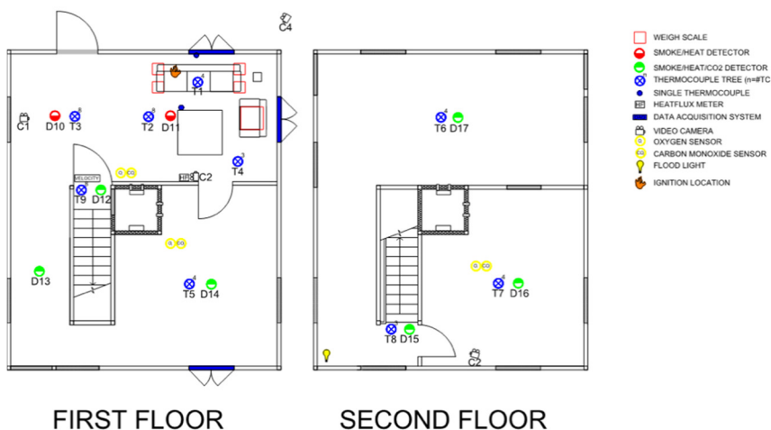
Fig. 1. Floor plan of the large scale test facility.
