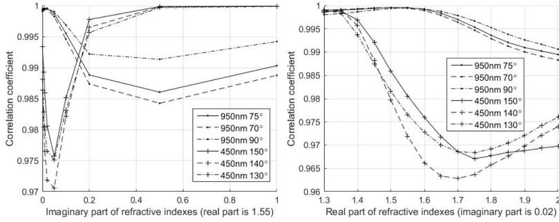
Fig. 3. The correlation coefficient of particle surface area concentration versus: (a) imaginary part of refractive indexes; (b) real part of refractive indexes.
