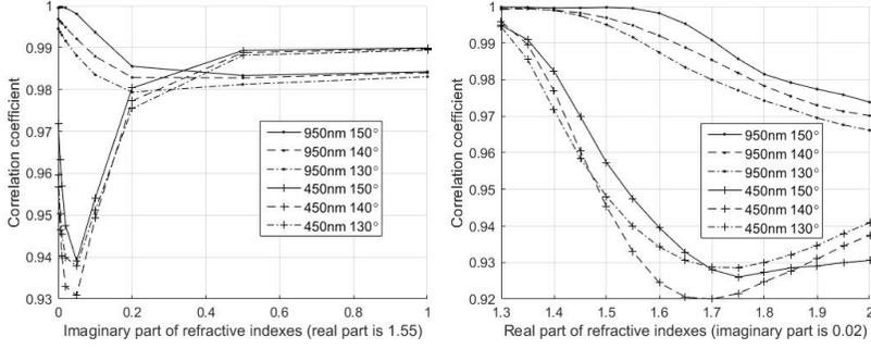
Fig. 2. The correlation coefficient of particle volume concentration versus: (a) imaginary part of refractive indexes; (b) real part of refractive indexes.
