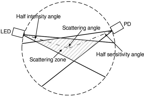
Fig. 1. Diagram of a practical photoelectric smoke detector.
