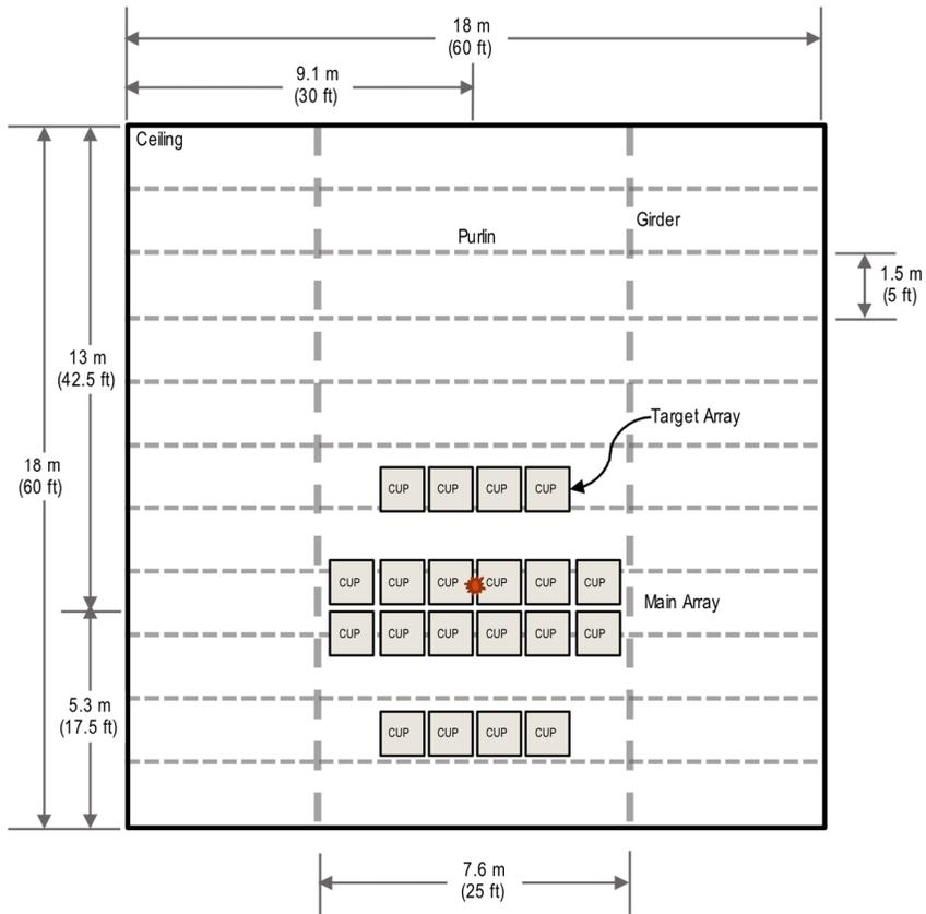
Fig. 2. Plan view of test configuration.
