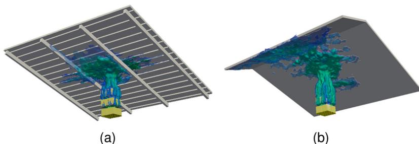
Fig. 1. FireFOAM simulations of ceiling interactions for an inclined ceiling (a) with purlins and girders; and (b) with a ridge [9].
