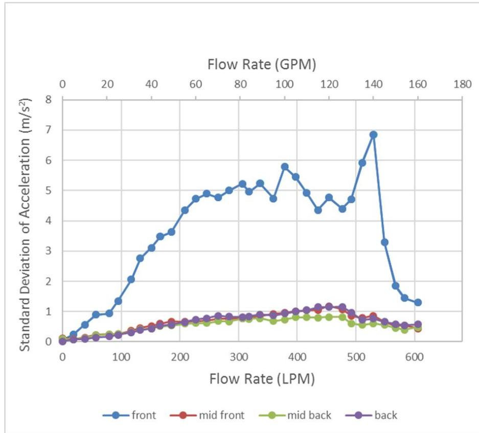
**Fig. 3.** Typical results of the standard deviation of acceleration versus flow rate for the four accelerometers. Data among the 50 consecutive runs was similar and therefore for visualization purposes only one run was used to represent all the data in the figure.
