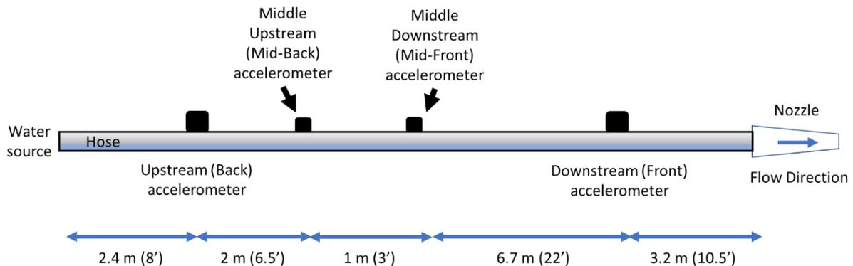
**Fig. 2.** The four accelerometer locations along the approximately 15 m (50 ft) long fire hose.
