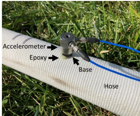
**Fig. 1.** The accelerometer attached to a base that was epoxied to the exterior fabric of the fire hose at the downstream (Front) location.
