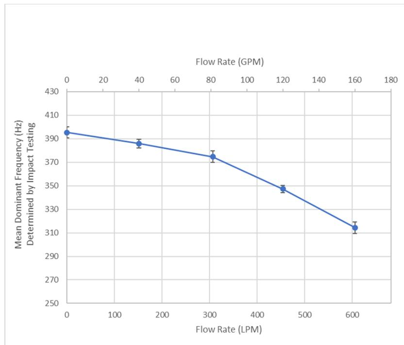
**Fig. 5.** The mean and standard deviation for the dominant frequency versus flow rate for the Front accelerometer from the impact testing.
