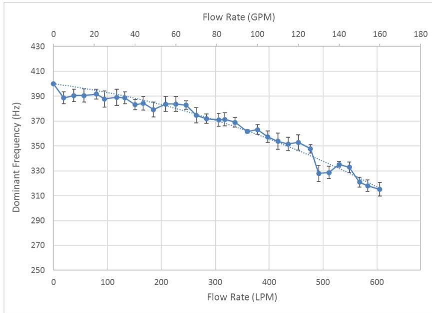
**Fig. 4.** The mean and standard deviation for the dominant frequency versus flow rate for the Front accelerometer from the flow-rate testing.
