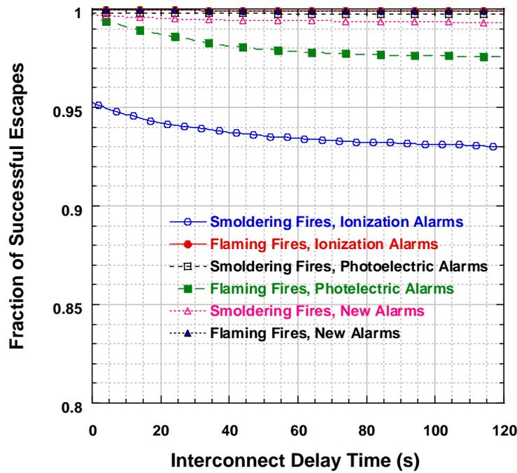
Figure 2. Case 2 - No smoke alarm in RFO and occupant of interest located outside RFO but not in room with the first responding smoke alarm.
