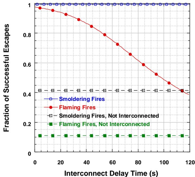
Figure 3. Case 3 - Smoke alarm located in RFO and occupant needing rescue located in RFO.
