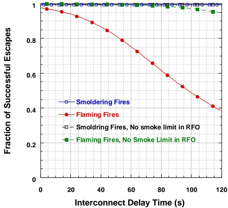
Figure 4. Comparison of results with and without a smoke limit in the RFO. Case 3 - Smoke alarm located in RFO and occupant needing rescue located in RFO.
