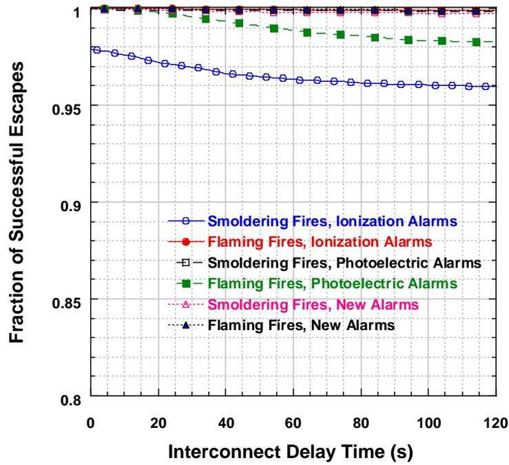
Figure 1. Case 1 - Smoke alarm in RFO and occupant of interest located outside RFO.
