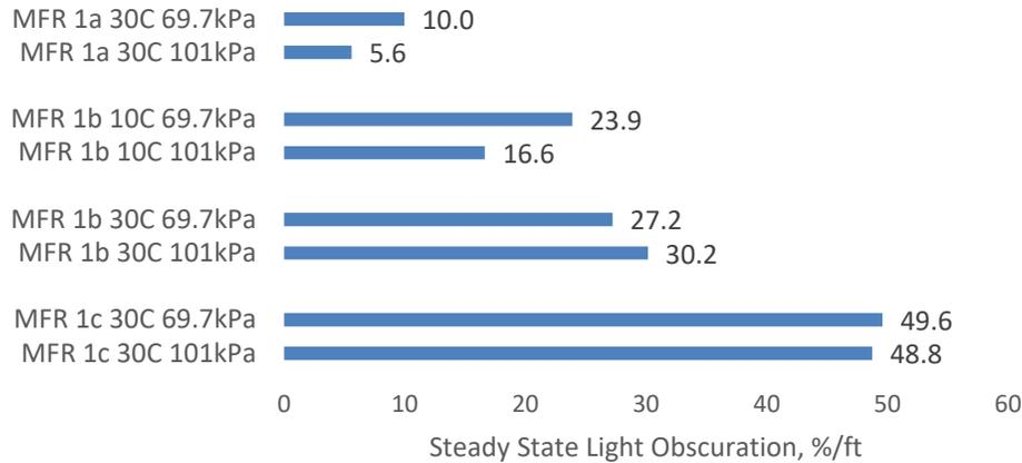
Figure 8. Varying Ambient Pressure and Smoke Generator Aerosol Production
