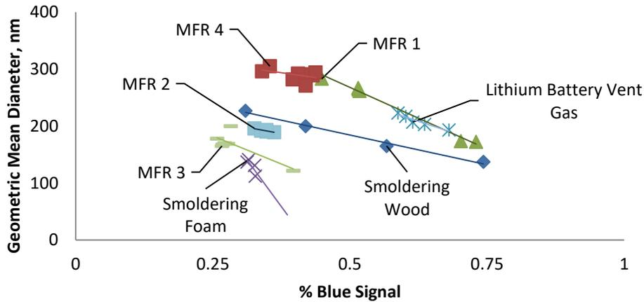
Figure 2 LSM %Blue Signal vs SMPS Diameter
