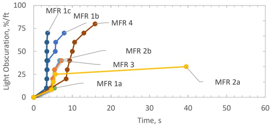
Figure 4 Time vs Light Obscuration for Transient Light Obscuration
