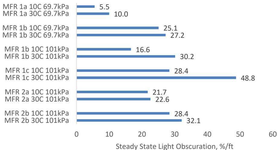
Figure 7. Varying Ambient Temperature and Smoke Generator Aerosol Production
