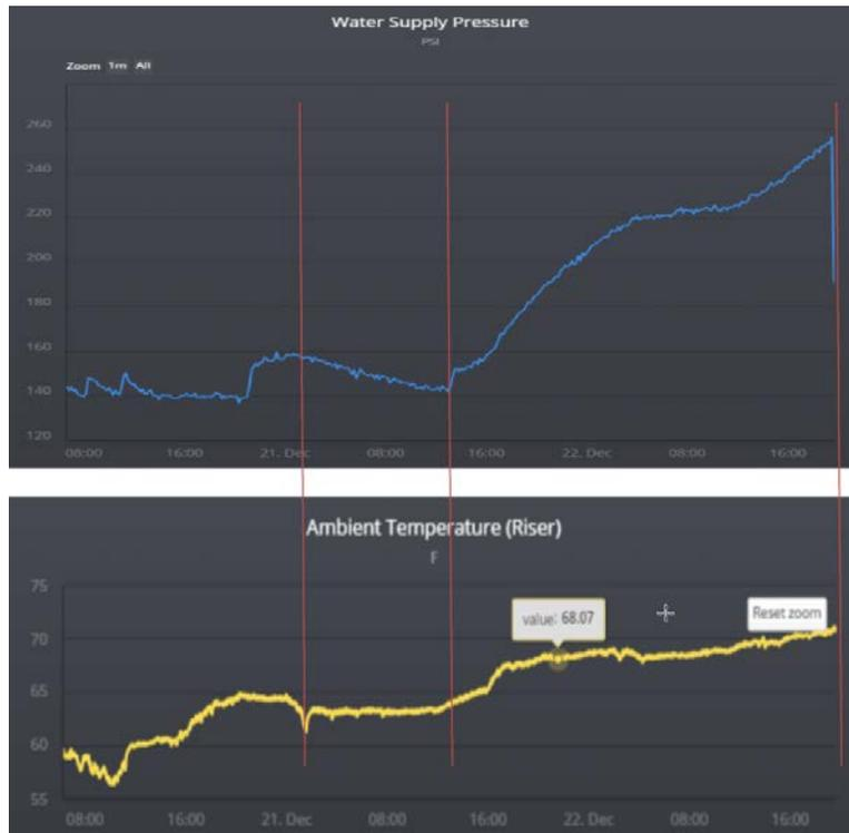
Figure 4 – Water pressure data vs. temperature data
