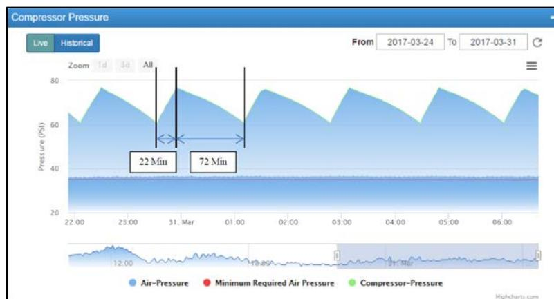
Figure 5 – Compressor pressure data over time
