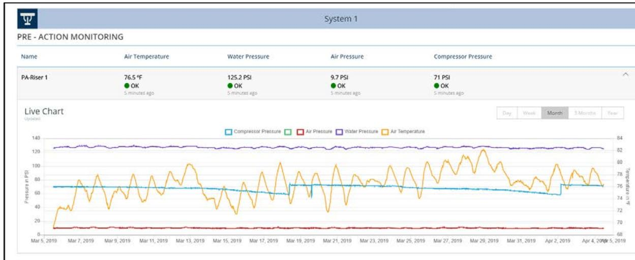
Figure 2 – Example of continuous data on a pre-action system as seen on the online user dashboard
