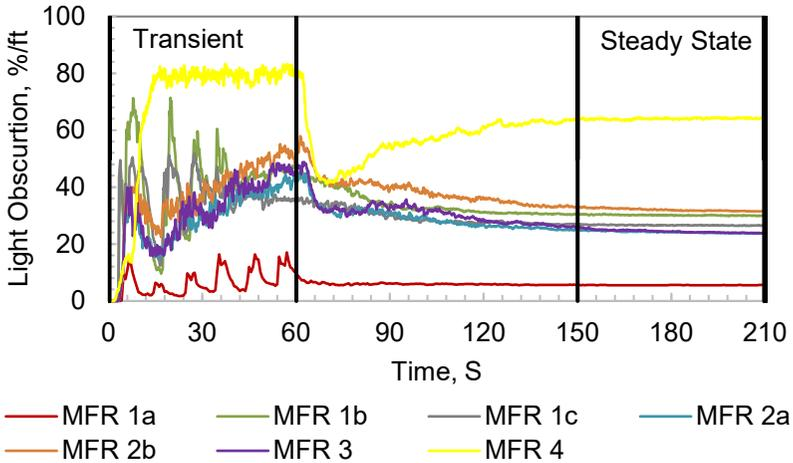
Fig. 1. Light obscuration vs time of individual tests.
