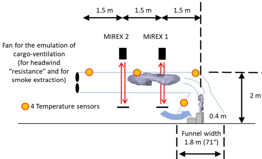
Fig. 11. Horizontal velocity test apparatus.
