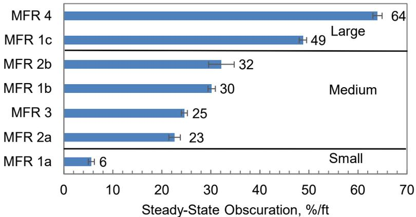
Fig. 3. Steady-state light obscuration by manufacturer.
