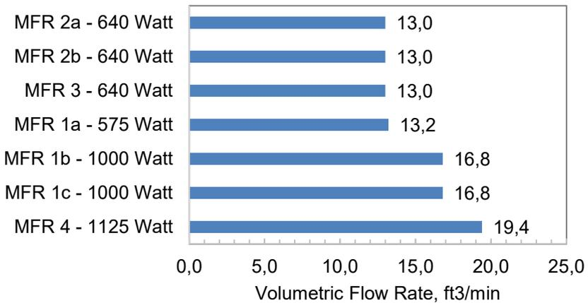
Fig. 5. Volumetric flow rate for smoke generators.
