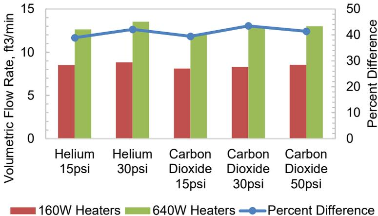
Fig. 8. Varying heater wattage.
